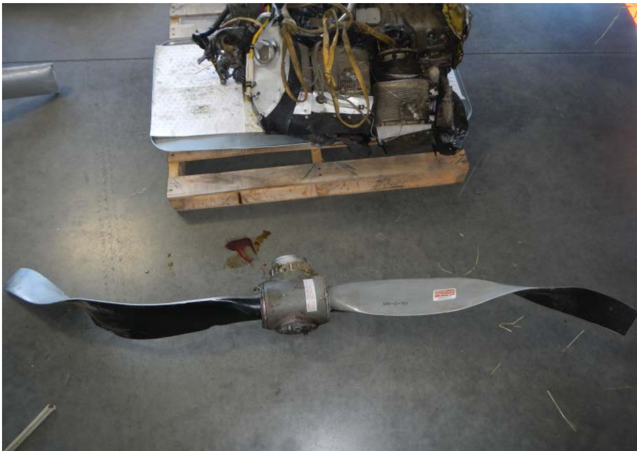
Figure 3 - picture of propeller blades (courtesy of Continental Motors, Inc.)
