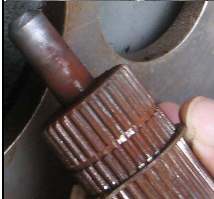
These two photos of George Adkin's splined shaft and adaptor show little or no wear... indicating good alignment between gearbox and engine.
