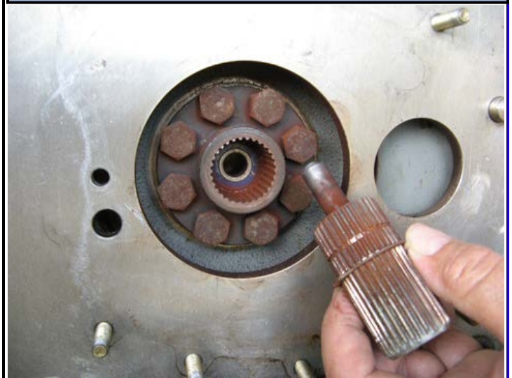
These two photos of George Adkin's splined shaft and adaptor show little or no wear... indicating good alignment between gearbox and engine.
