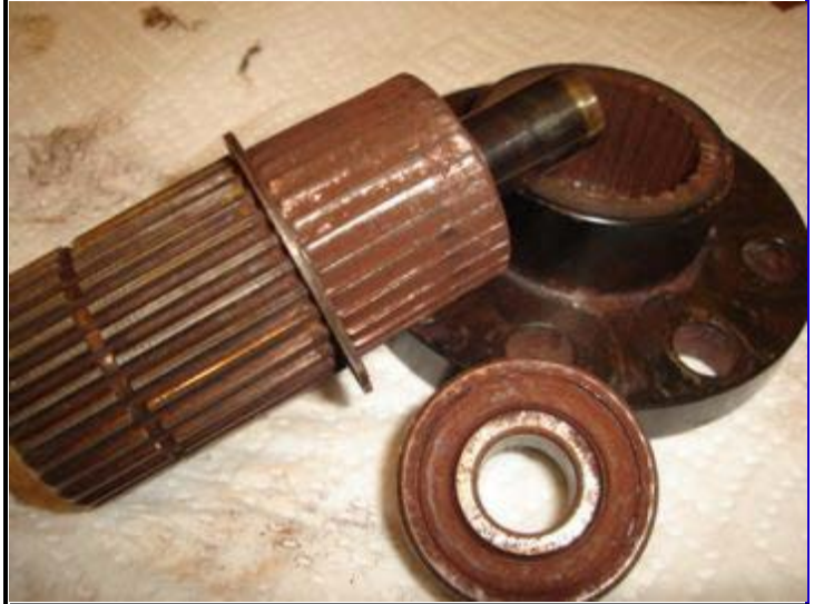
Above photo is Bill Yamokowski's splined shaft, his splined shaft adapter, and his splined shaft pilot bearing. The left half of the shaft, which goes into the gearbox looks okay. The right end, which goes into the adaptor plate has its spline stripped and worn down. It free-wheeled in the adaptor plate, causing the prop to stop producing thrust.
