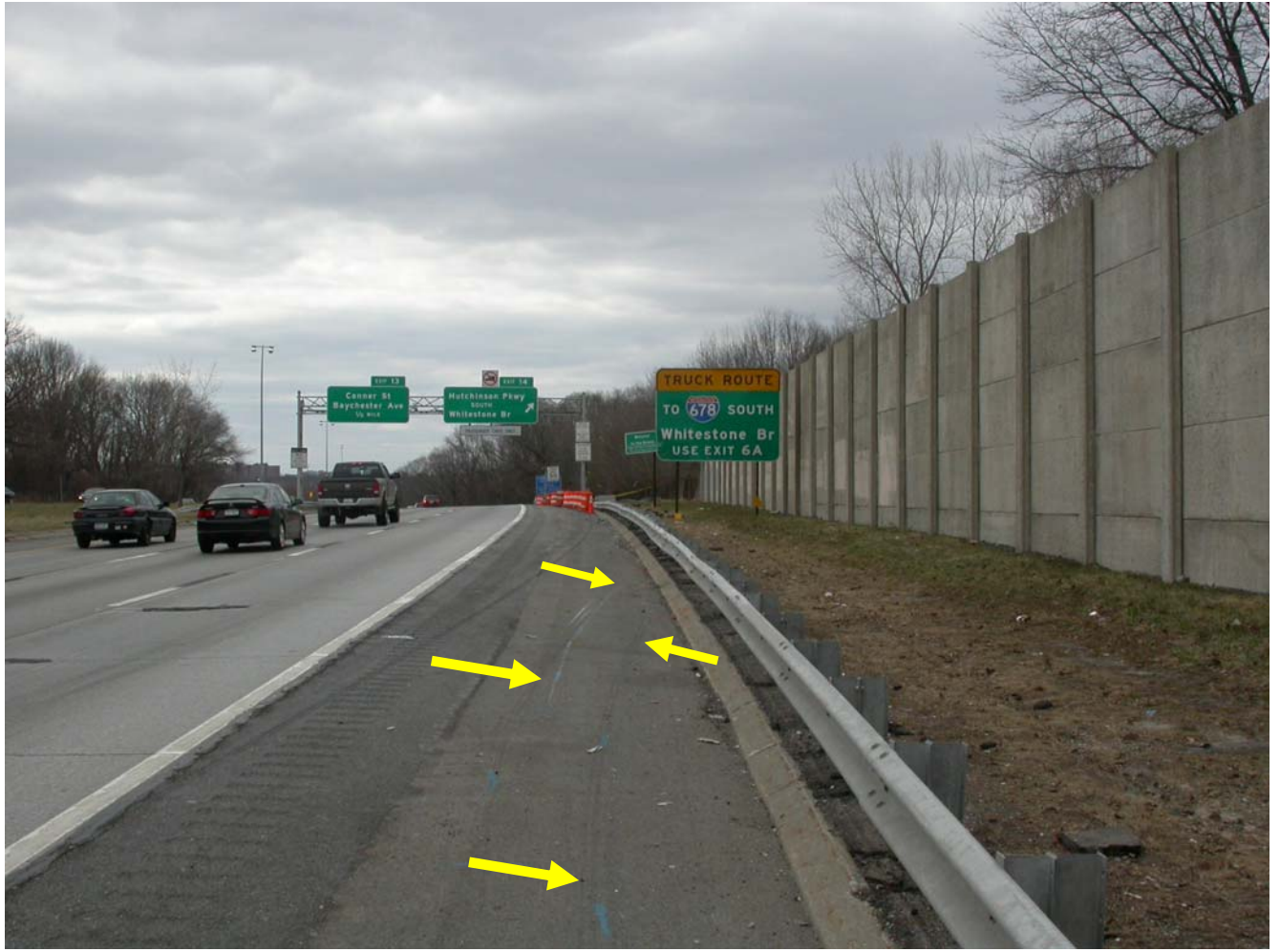
Figure 4 – Arrows highlight the physical evidence indicating the path of the bus as it veered back towards the guardrail and impacted the guardrail for a second time. (Unless indicated by an arrow, tiremarks and scrapemarks shown in the photograph are not associated with this accident.)
