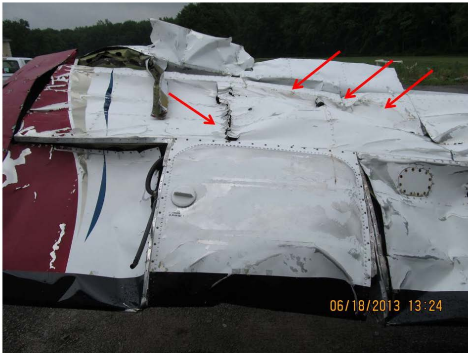
Photo 14 - Outboard portion of right wing. The left arrow shows an area of compression damage to the upper service of the right wing. The series of arrows highlight a diagonal wrinkle across the top of the right wing. The wing skins on each side of the tank are compressed downward. The tank wing skin is compressed downward around the stringers.
