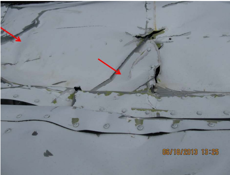
Photo 18 - Diagonal wrinkles and compression damage to the top of the right wing.
