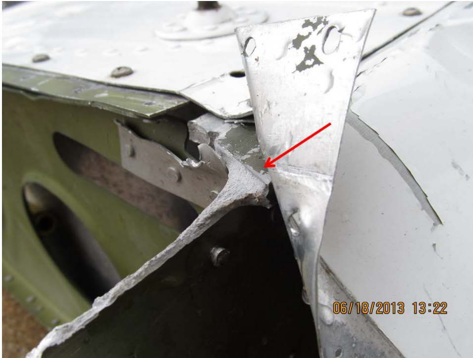
Photo 7 - The lower spar cap exhibits characteristics of tension overload.
