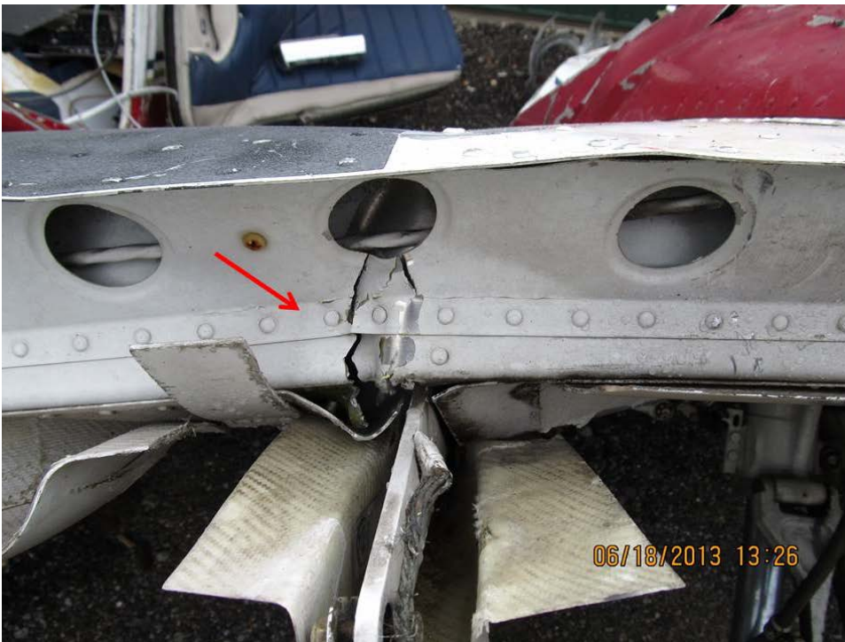
Photo 20 - Compression damage to lower cap of rear spar.
