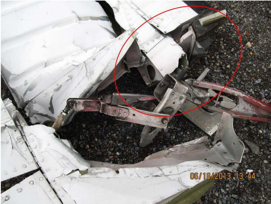
Photo 25 - The highlighted area shows the main spar of the stabilator.
