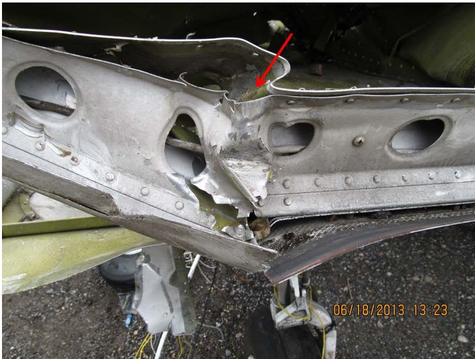
Photo 8 - The section of the rear spar is buckled at the top.
