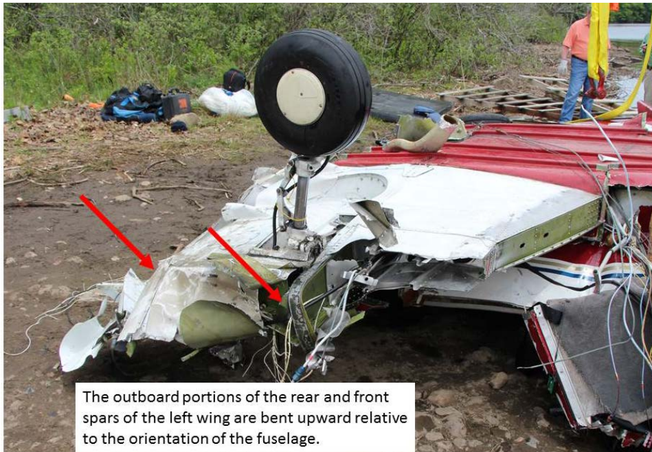
Photo 1 - The front and rear lower spar caps of the left wing are bent in an upward direction. The fuselage and right wing (still attached) impacted the water inverted.
