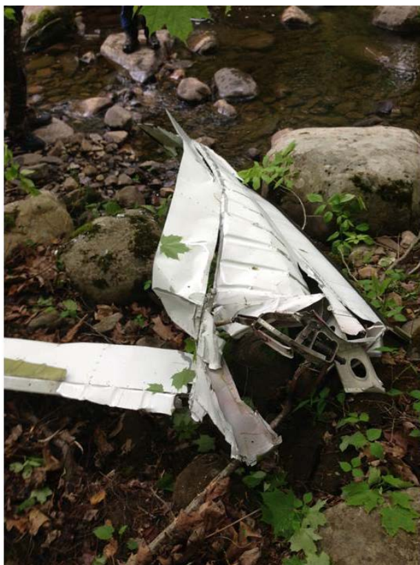
Photo 24 - Another view of the left stabilator displaying the downward bend.
