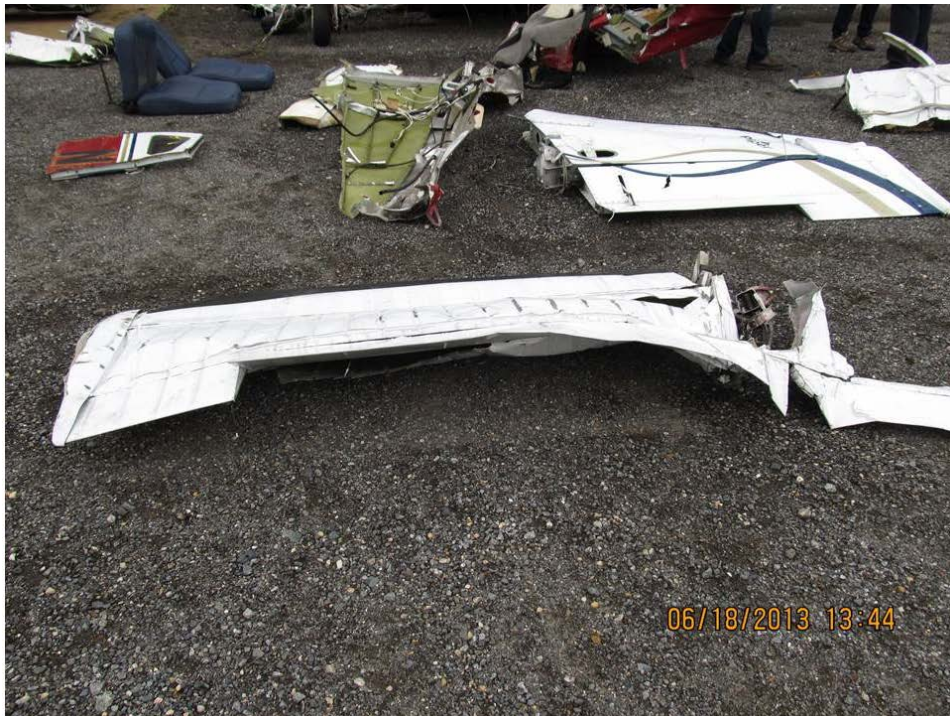
Photo 23 - The left stabilator exhibits a downward bend.
