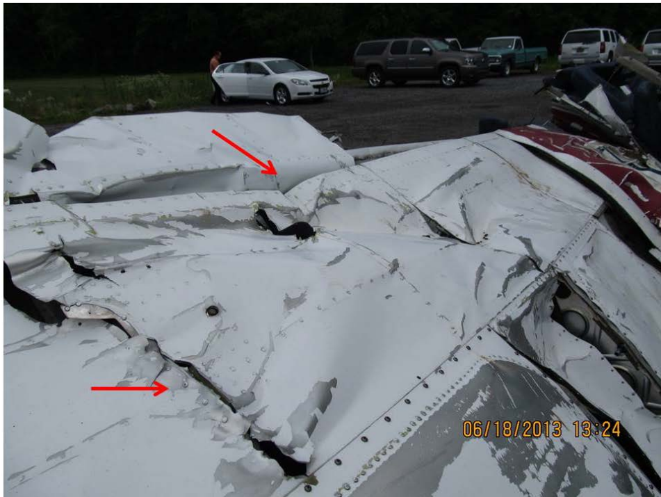
Photo 16 - The arrows highlight compression damage on the upper surface of the right wing. The diagonal wrinkle is also visible.
