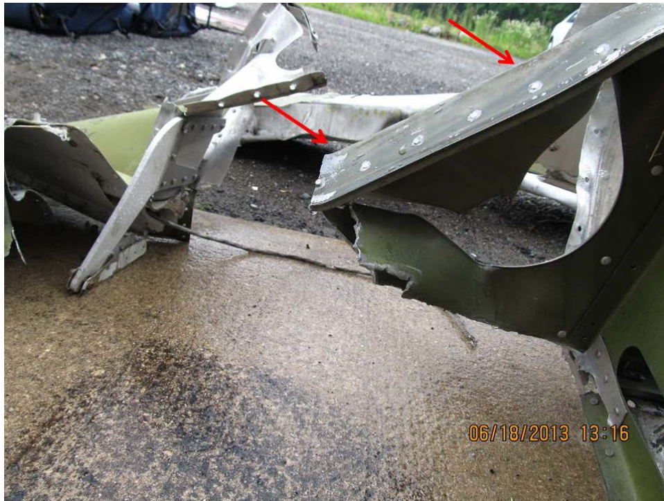
Photo 6 - Reflex bend of upper spar cap.
