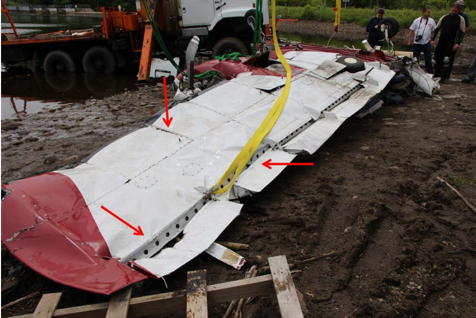
Photo 13 - The right wing is inverted. The arrows pointing to the aft spar highlight points of compression damage to the bottom of the aft spar (r) and the top of the aft spar (l).
