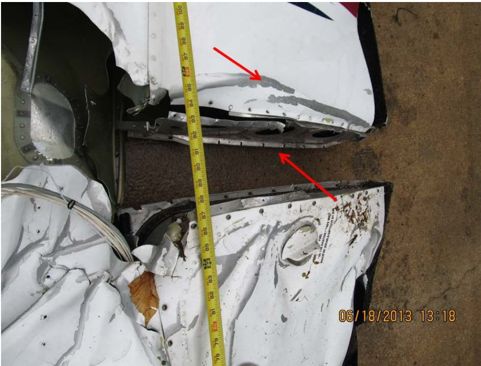
Photo 12 – An arrow highlight the compression wrinkles on the top skin of the left wingtip. The other arrow highlights the tension tears at the rivet holes on the bottom skin.
