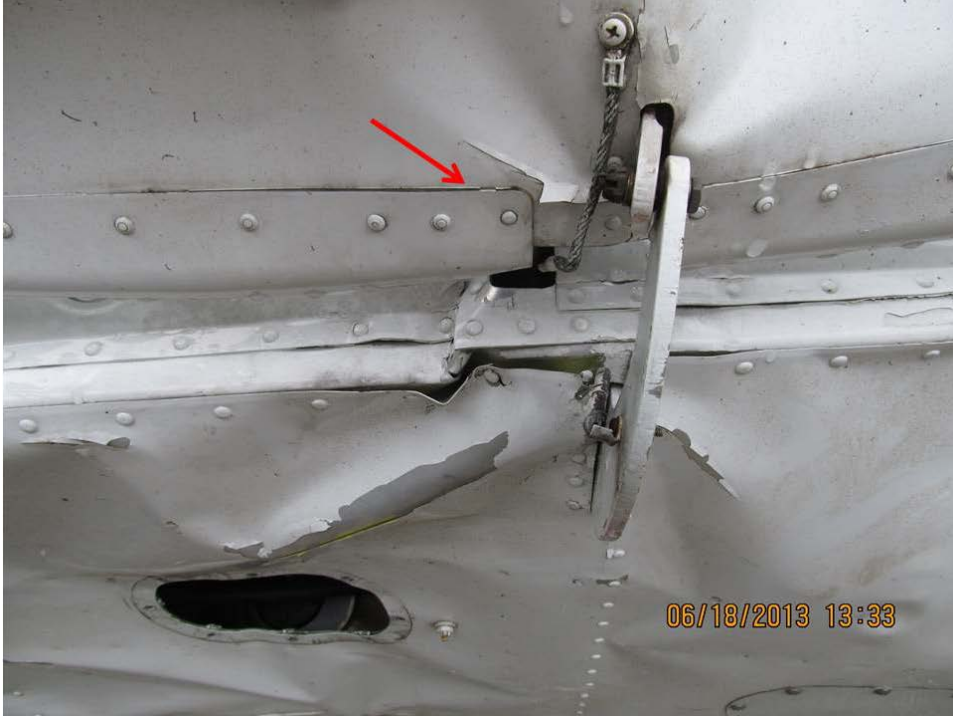
Photo 21 - Compression damage at lower cap of rear spar.
