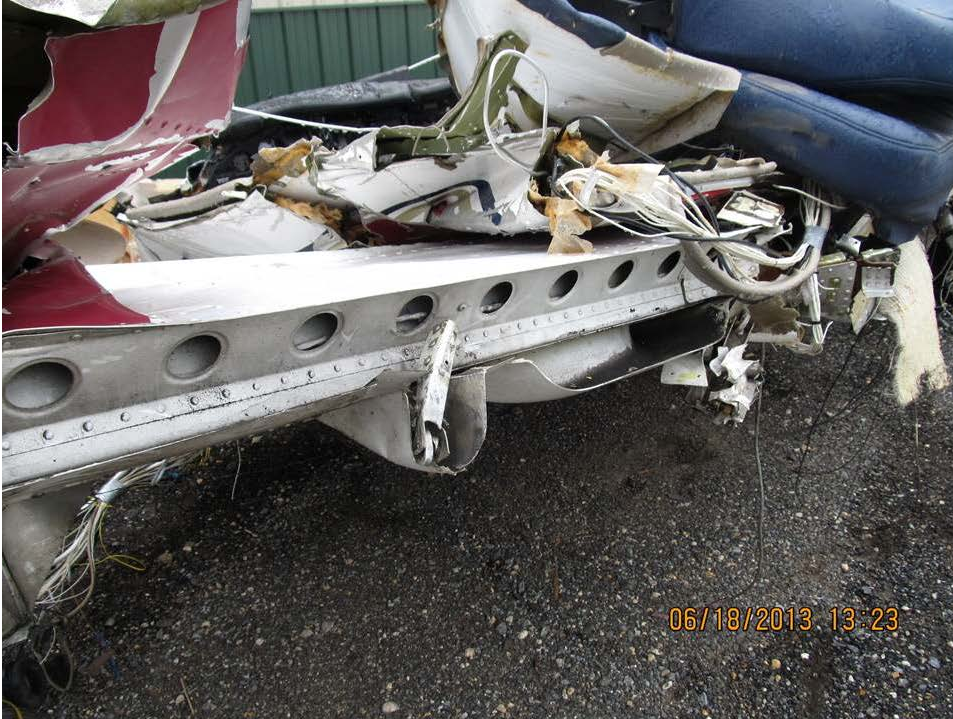
Photo 9 - A large portion of the rear spar is relatively free from distortion.
