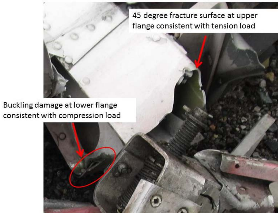
Photo 26 - The upper portions of the stabilator spar exhibit 45 degree fracture surfaces. The lower surfaces are buckled.
