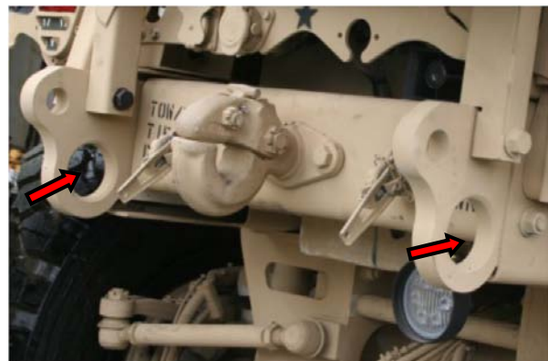
Figure 3: Aft Tiedown Provisions
