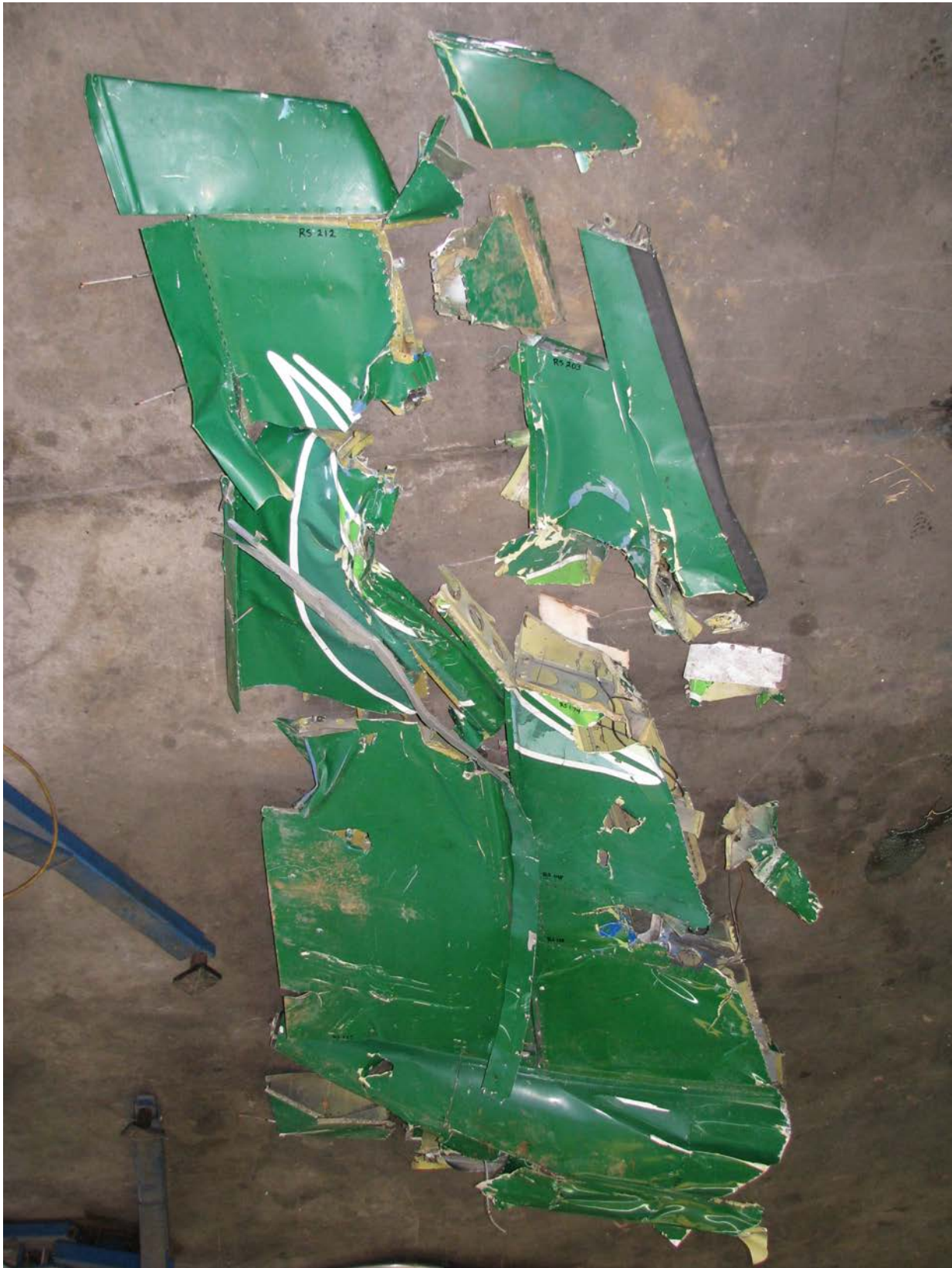
Figure 12 – Vertical stabilizer and rudder damage
