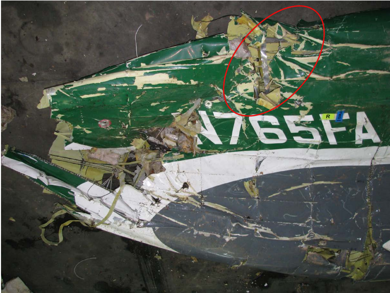
Figure 11 – Right fuselage damage oriented diagonally
