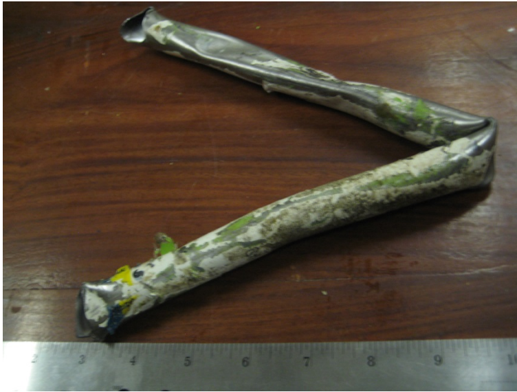
Figure 55 - Hydraulic System 2 Hydraulic Line
