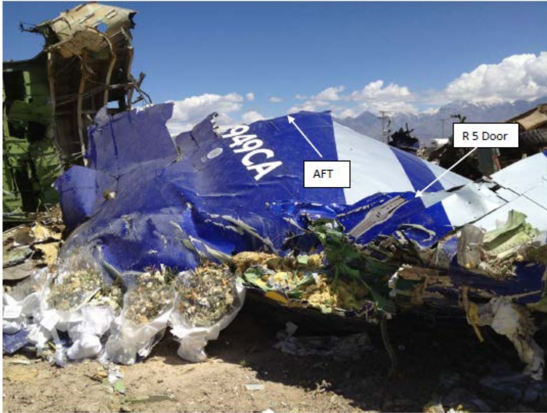
Figure 7 - FUSE-1 Panel Section
