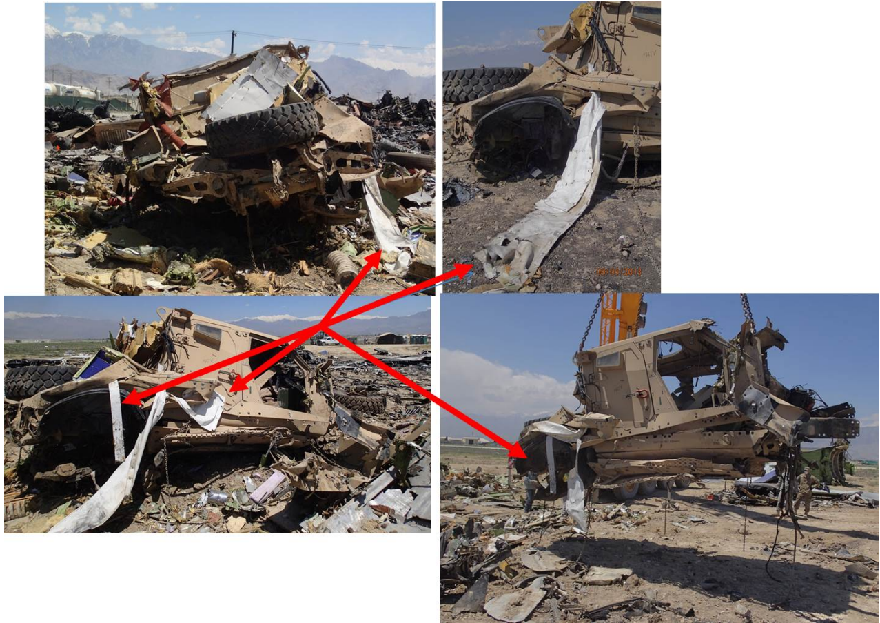
Figure 43 - Trapped APB Liner Material (1)
