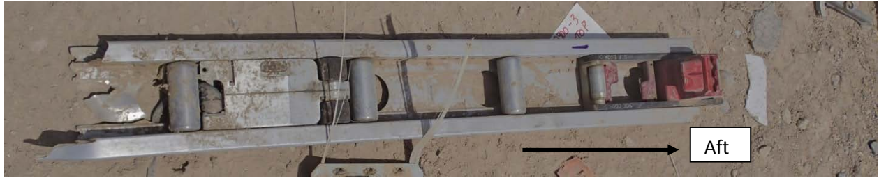
Figure 17 – N949CA Fixed End Stop (1) (part number 289100-3)
