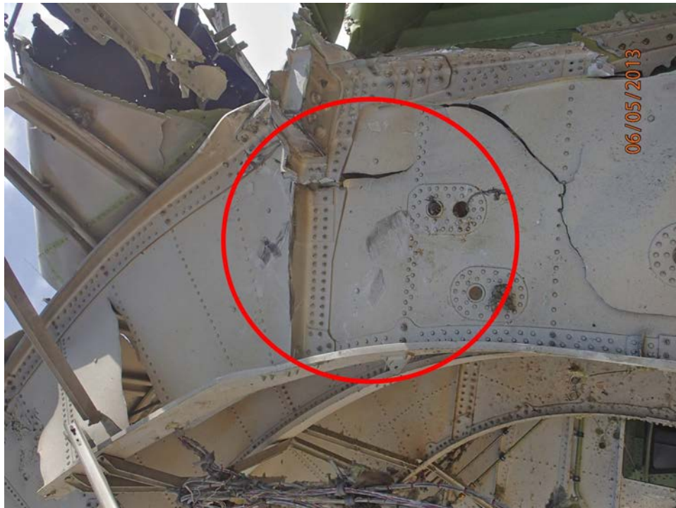
Figure 77 - Frame at STA 2412 Black Tire Transfer
