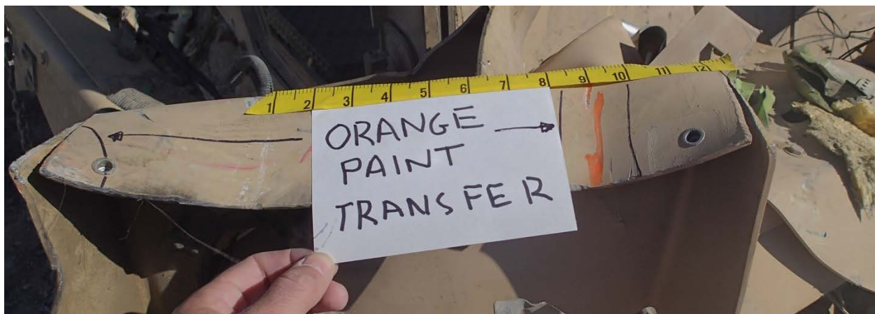
Figure 40 - Orange Paint Transfer (1) to M-ATV
