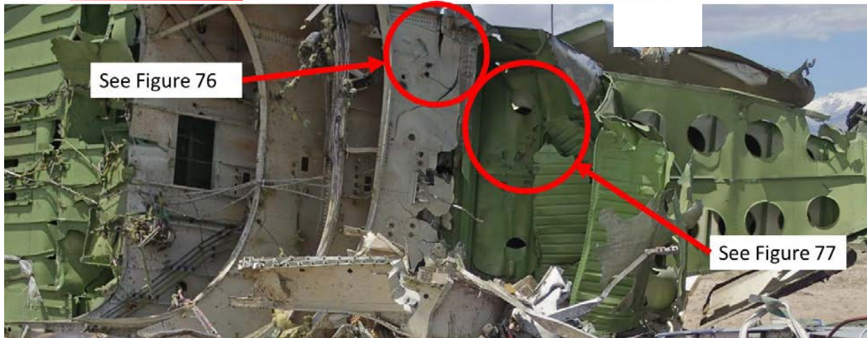
Figure 76 - Lower Side of the VTP Structure with Black Tire Transfer Marks at STA 2412
