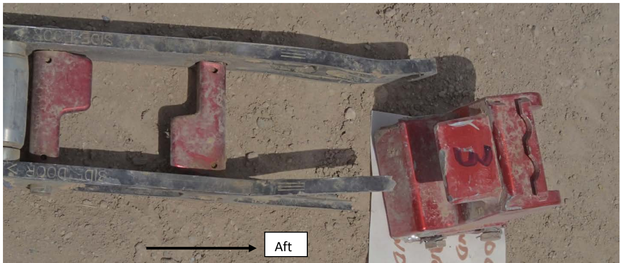
Figure 19 – N949CA Fixed End Stop (3) (part number 289100-3)
