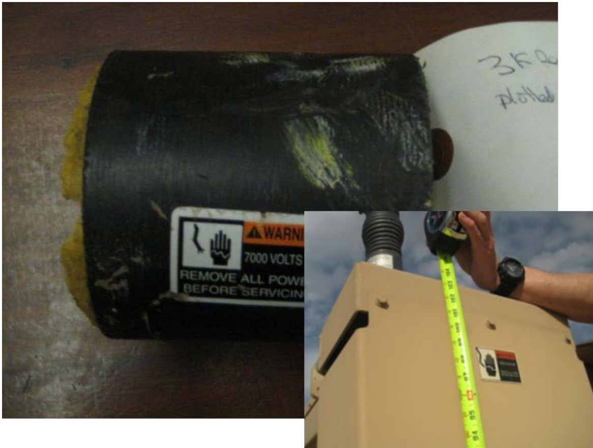
Figure 56 - M-ATV Antennae Component Recovered from the Runway
