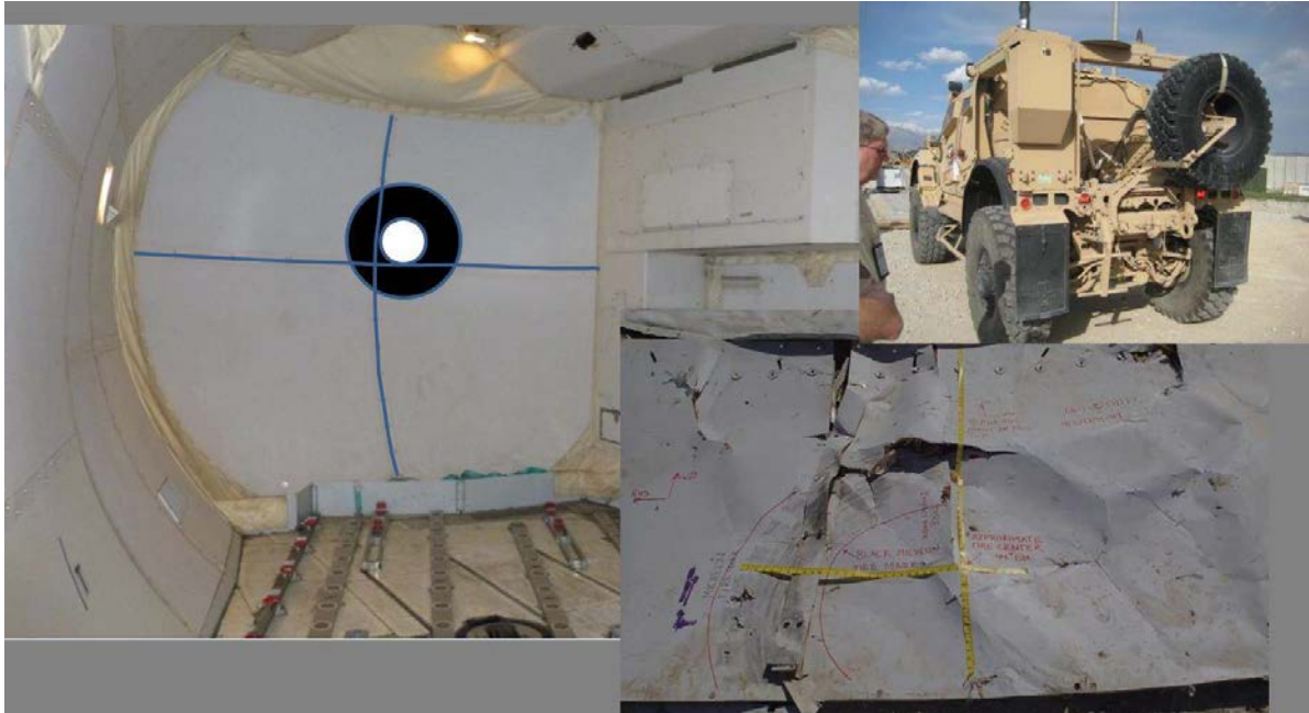
Figure 58 - APB Cargo Liner Tire Witness Marks
