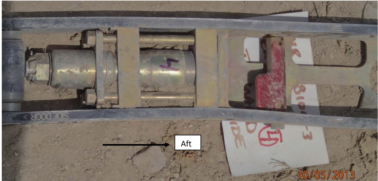
Figure 20 – N949CA Retractable End Stop Tray (4) with Missing End Stop (part number 288100-3)
