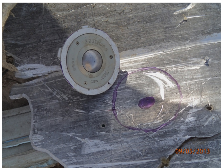
Figure 68 - Roller Bearing Witness Mark at 48 Inches
