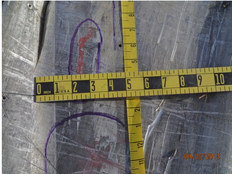
Figure 67 - 20 foot G code Pallet Red Paint Transfer Marks & Material Smearing.
