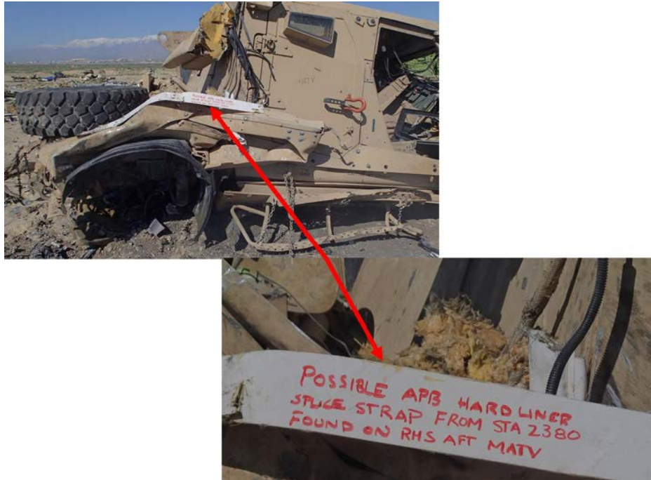
Figure 44 - Trapped APB Liner Material (2)
