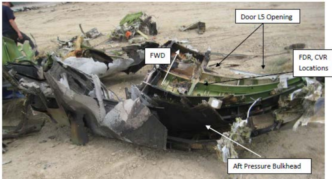
Figure 8 - FUSE-2 Panel Section
