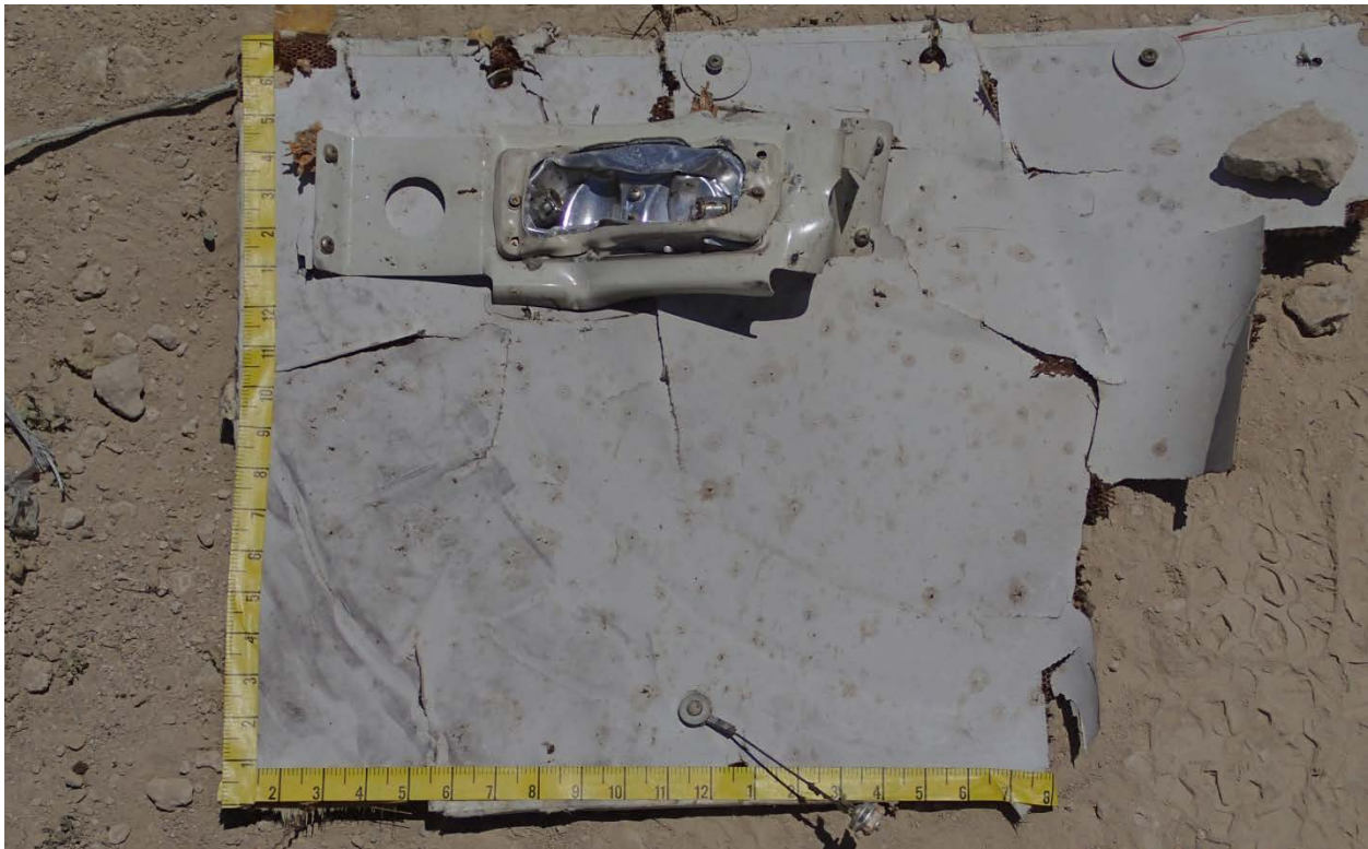
Figure 65 – Unidentified Panel with Interior Light Fixture & Grounding Cable
