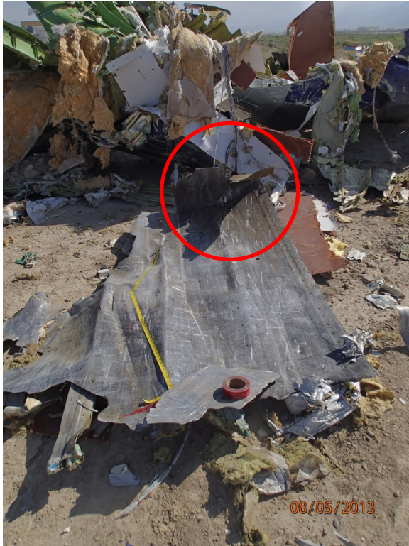
Figure 69 - Curled Deformation of a Partial G code Pallet
