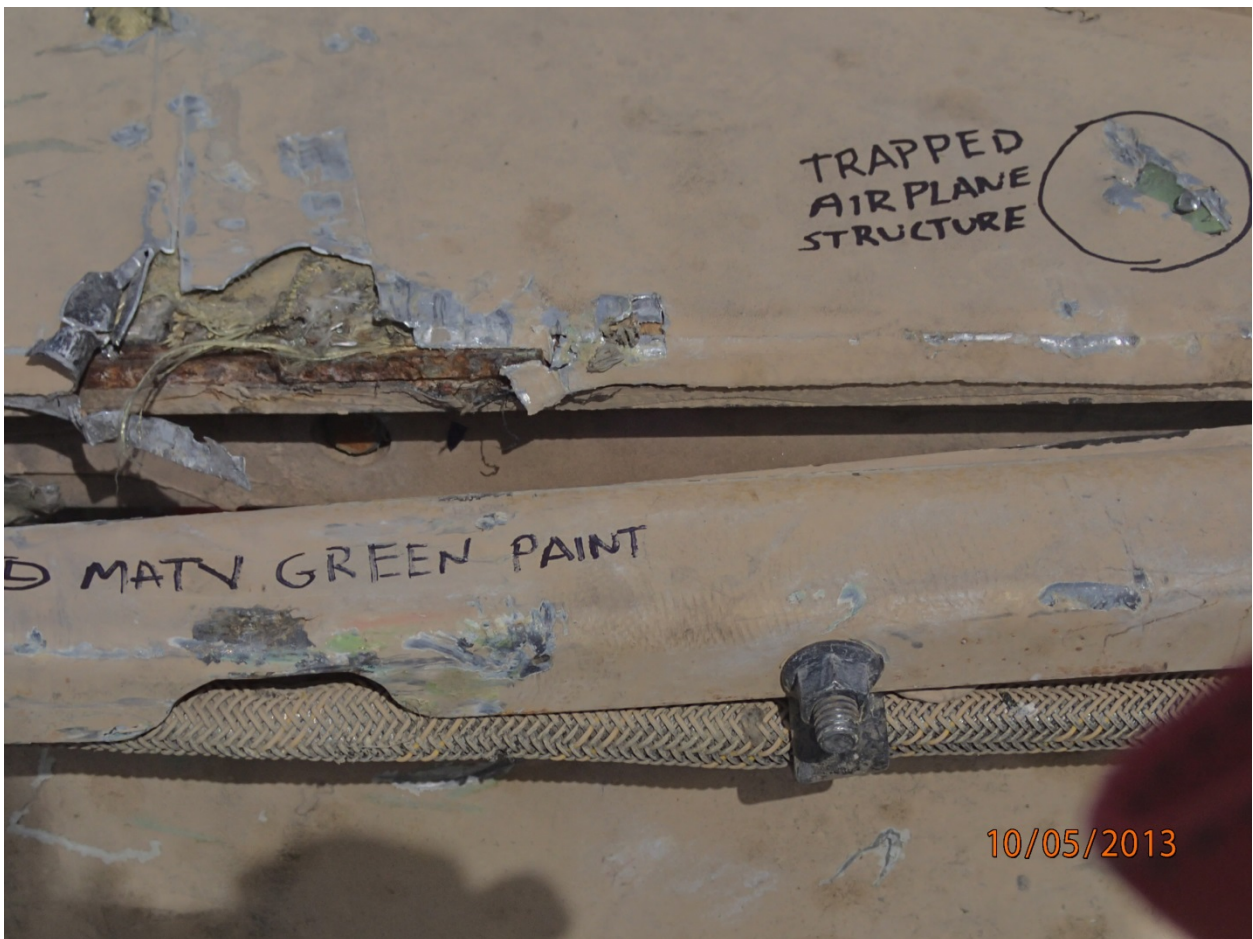
Figure 42 - Airplane Green Primer Paint Transfer on M-ATV
