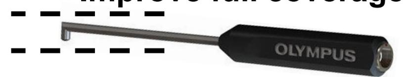
Right-angle probe has potential to lose contact with hole during inspection
