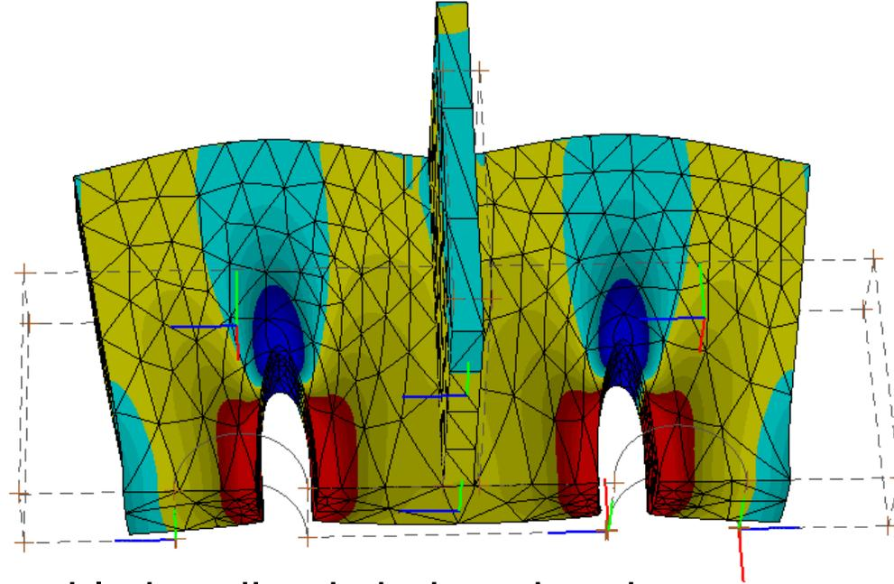
No noticeable bending is induced and stress/deformation around holes are symmetric.
