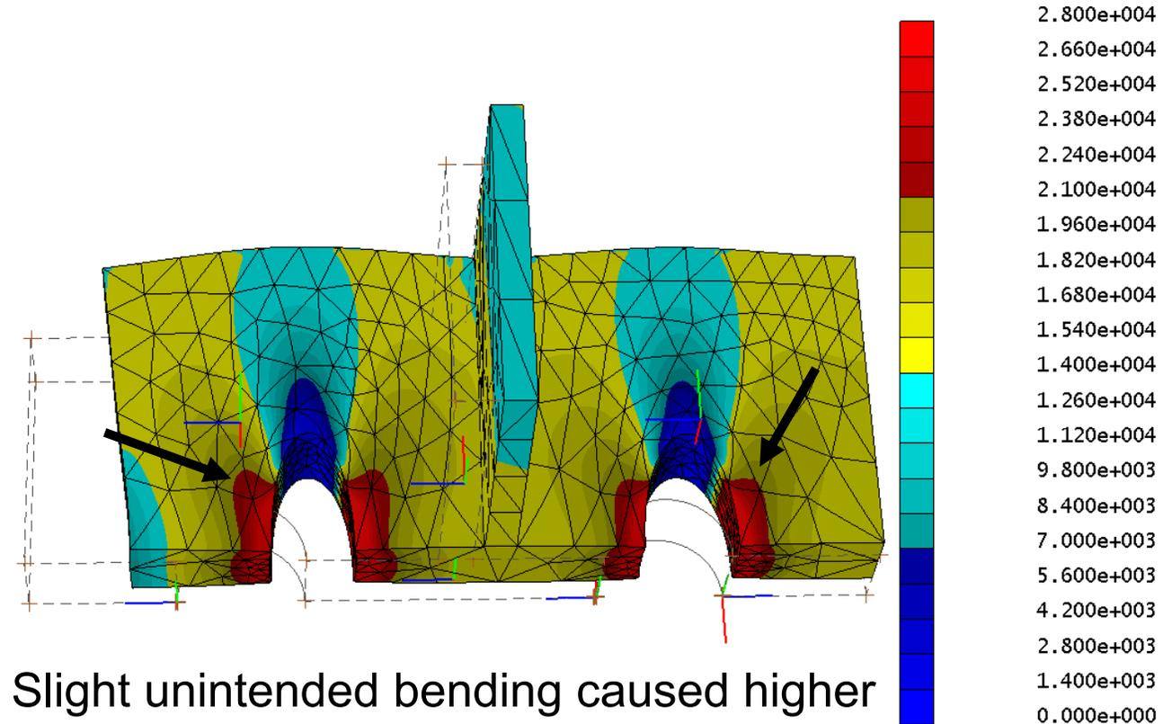
Slight unintended bending caused higher stresses on left side hole. The difference caused cracks to not grow analytically on the side closest to the constraint.
