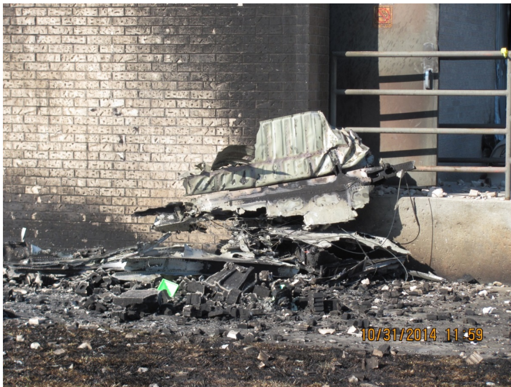
Photo 3 – Portion of left wing and flap at northeast corner
