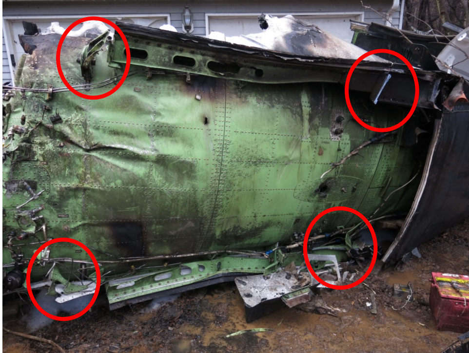
Figure 22. Center section of fuselage with wing attach fittings circled.
