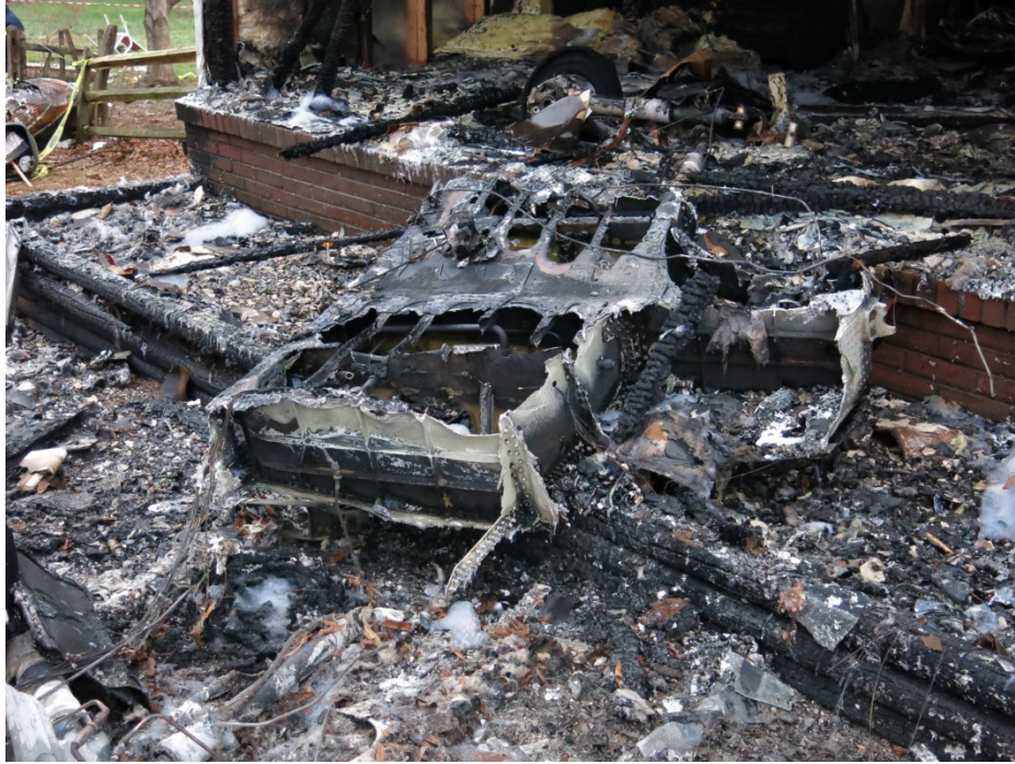
Figure 32. Wing center section, with left main landing gear inside of 19733 Drop Forge Lane.
