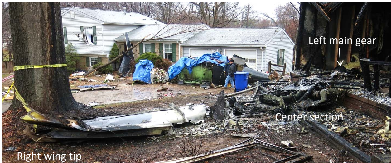
Figure 30. The remnants of the wing are shown in this photograph, which faces the leading edge. The house in the background is 19737 Drop Forge Lane and the fuselage is in front of the garage doors.
