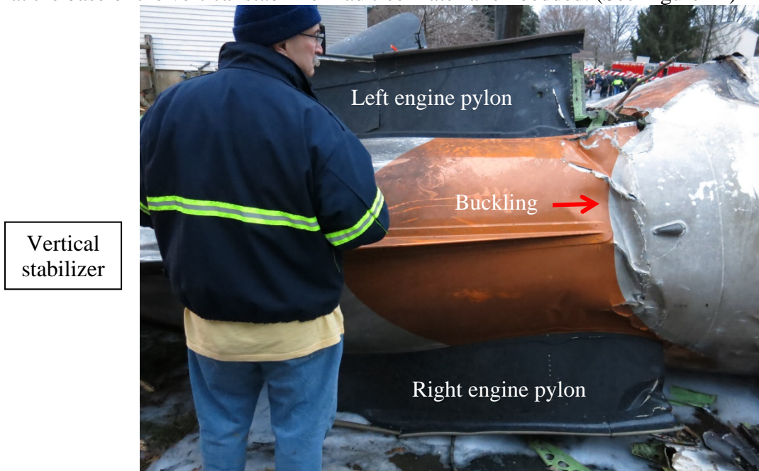
Figure 21. Compressive buckling in crown skin. This view looks down on the top of the crown.
