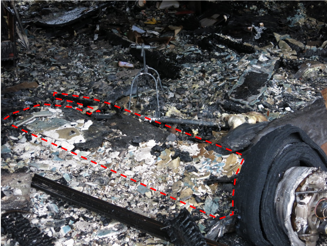
Figure 33. Dashed outline of the carbon fiber panel edges within the 19733 house, which are outboard of the visible left main landing gear tire. These left wing panels were similar to the accessible right wing panels which were above and ahead of the right wing flap.
