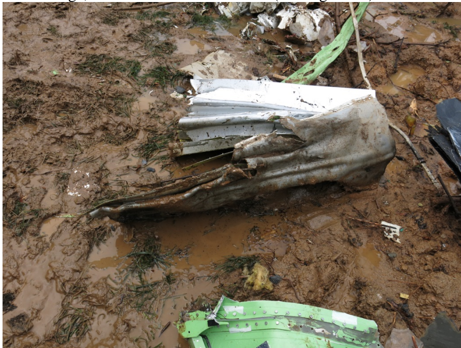
Figure 25. Three feet of left wing structure and aileron.
