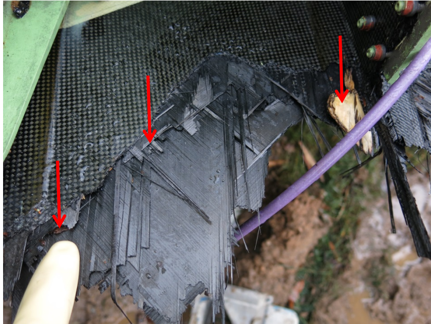
Figure 24. Embedded into the carbon fibers at the base of the vertical stabilizer were fragments of wood.
