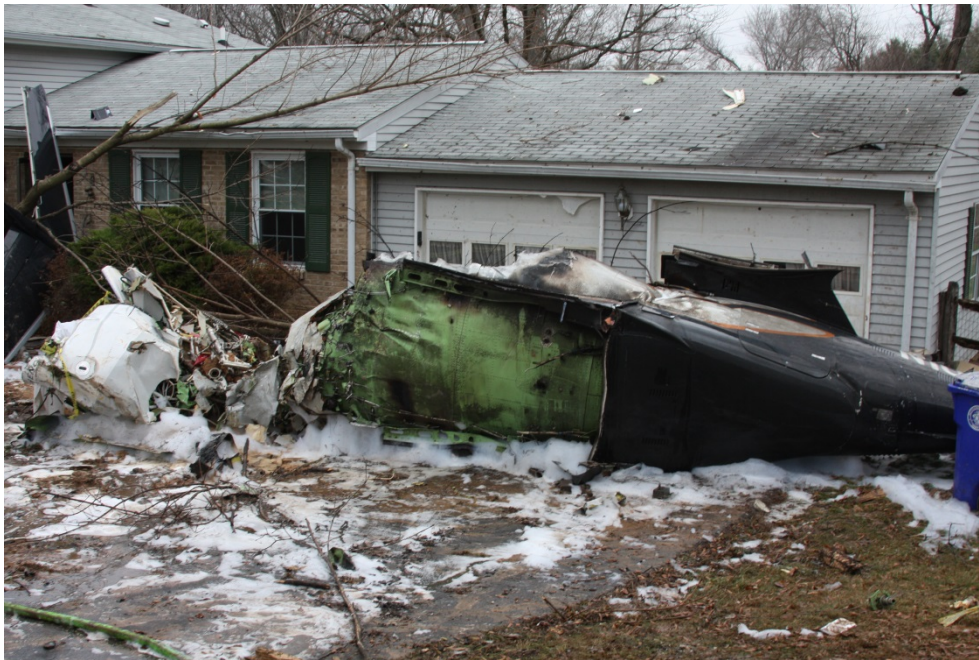
Figure 18. Fuselage in driveway of 19737 Drop Forge Lane. The belly of the fuselage folds upward forward of the green area, which had been above the wing.
