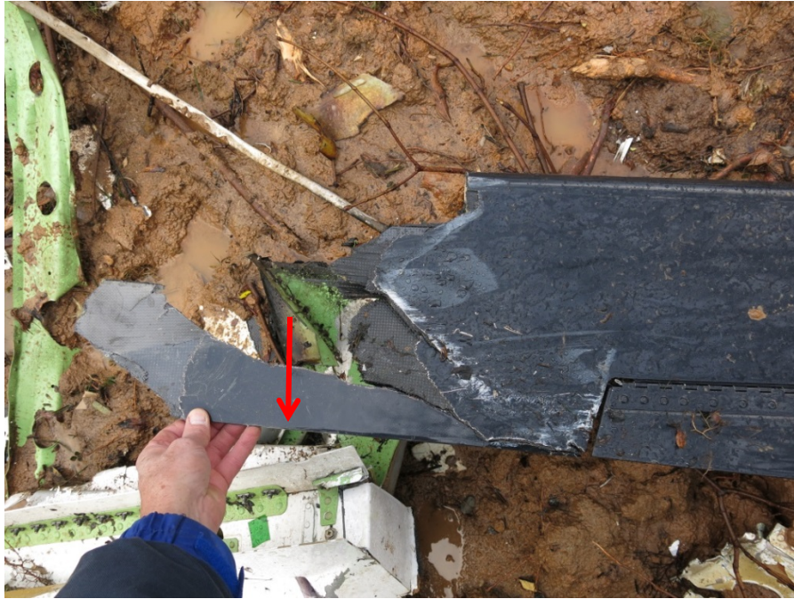
Figure 16. Carbon fiber trailing edge of elevator, found in wall of 19737 house.
