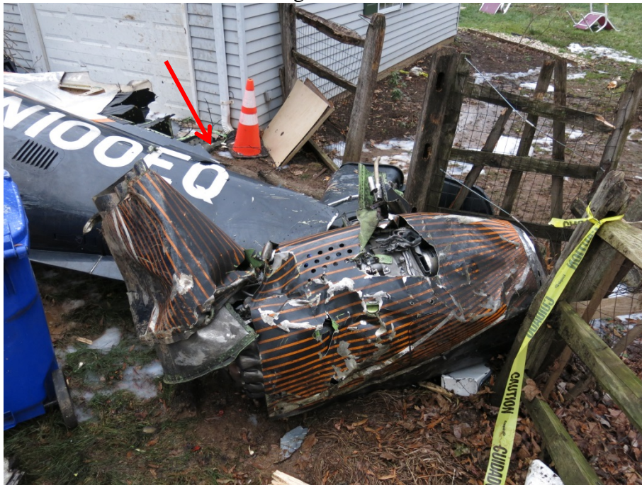
Figure 23. Tail cone and inverted left engine. The arrow orients where wood was embedded into carbon fibers at base of vertical stabilizer, as shown in Figure 24.
