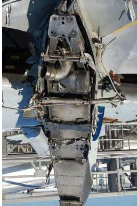
RH pylon attached to wing
