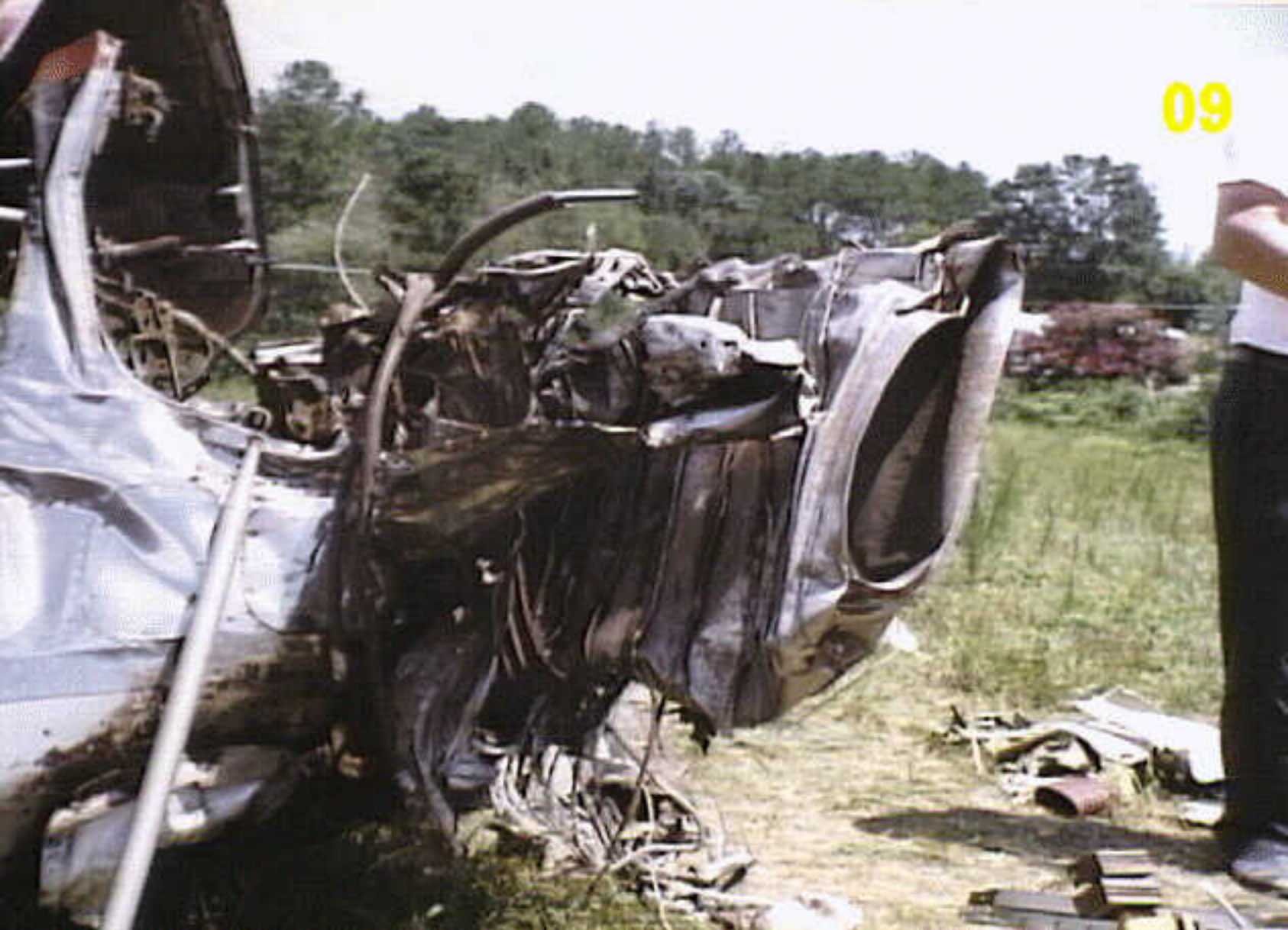
Structures 7A - Photo 09. Inboard, aft side of left nacelle skin.
