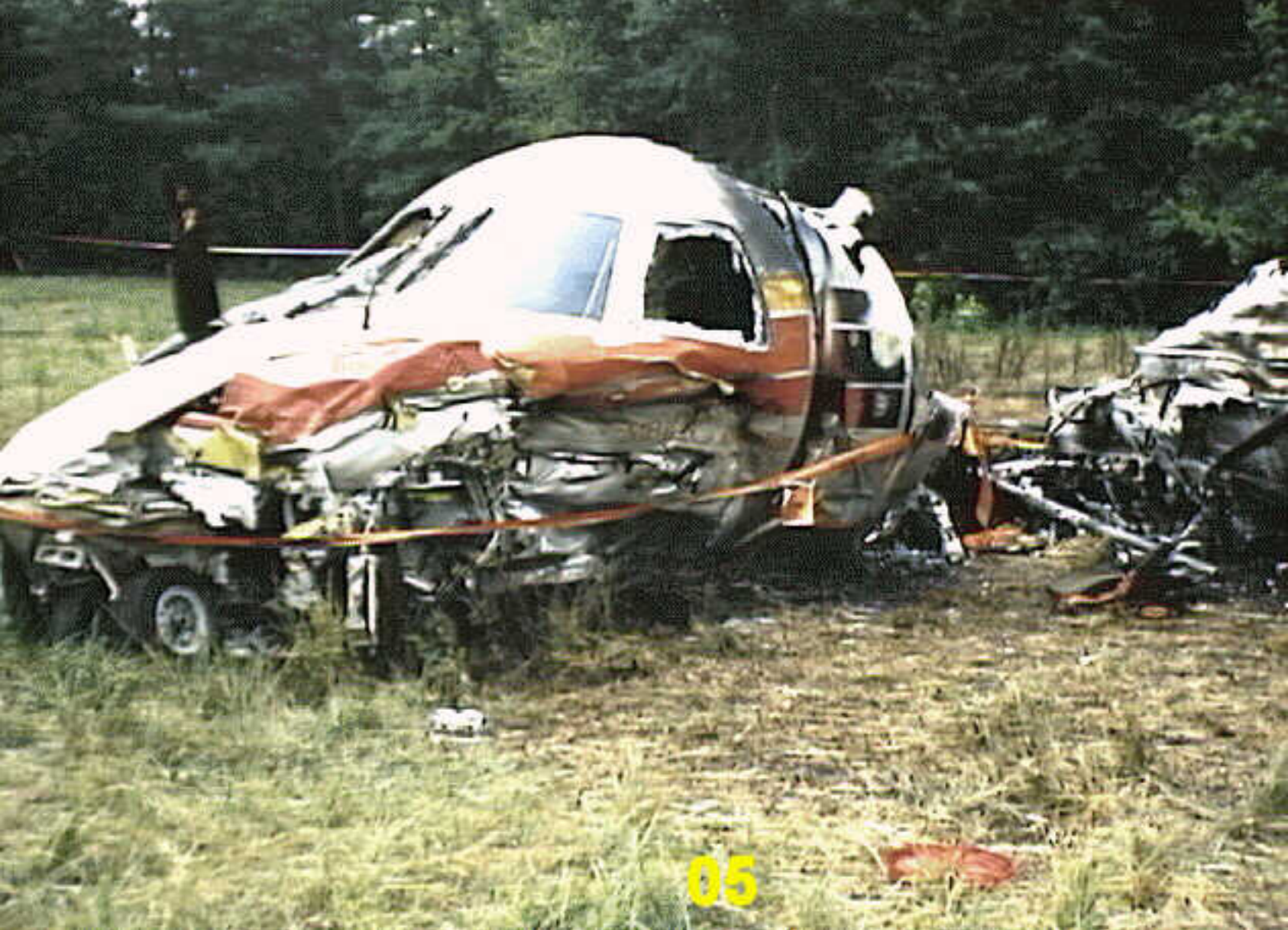
Structures 7A - Photo 05. Inward, upward crushing to left side of forward fuselage.
