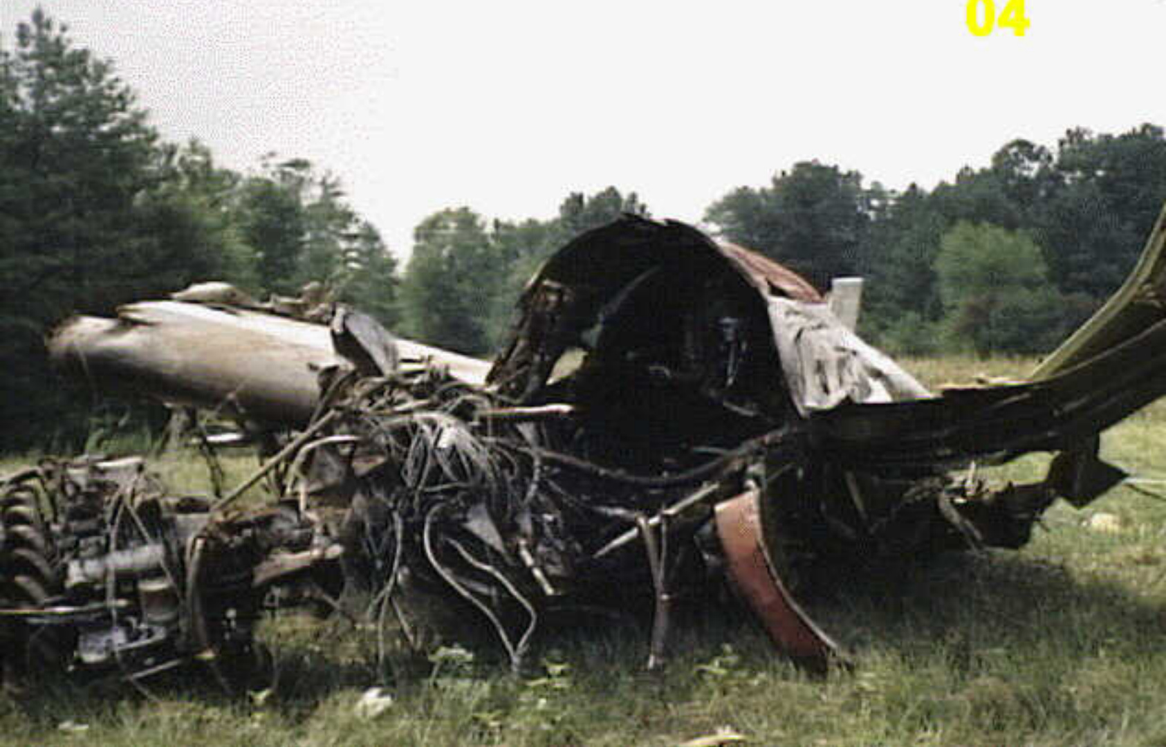
Structures 7A - Photo 04. Left engine and inboard section of left wing.
