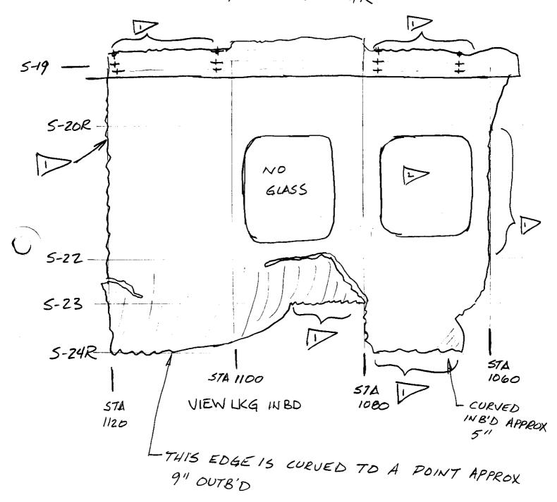
IN NET AREA FAILURE ALONG 'RIVET LINE'
