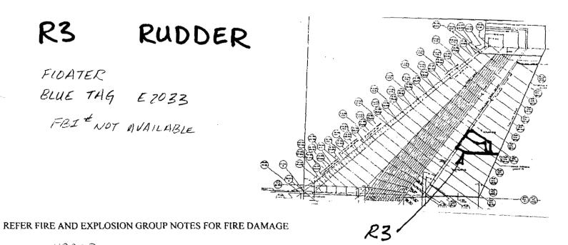
UPPER RUDDER SECTION MEASURING APPROX IMATELY 55" × 6° FROM RUDDER STATION 147.7 TO 207.6 RUNNING FROM LEADING EDGE TO TRAILING EDGE.
