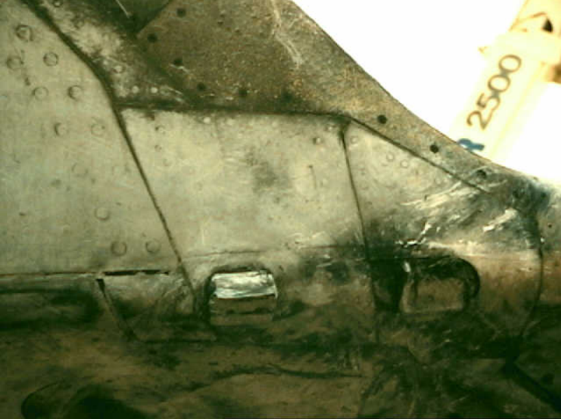
Structures 7 - Photo. 5 - View of the fractured lower right winglet attach fittings
