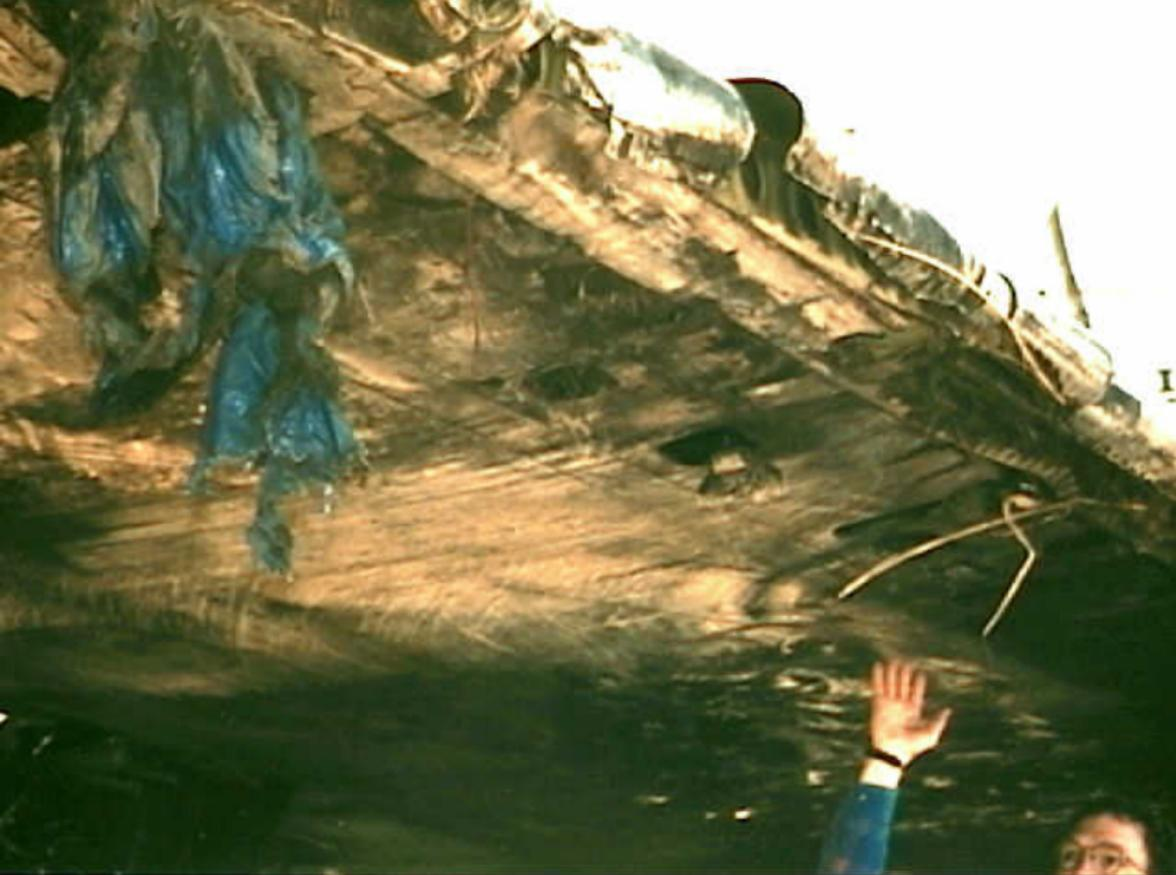
Structures 7 - Photo. 4 - View of right wing leading edge number 8 slat Note: interior structure is embedded with vegetation.
