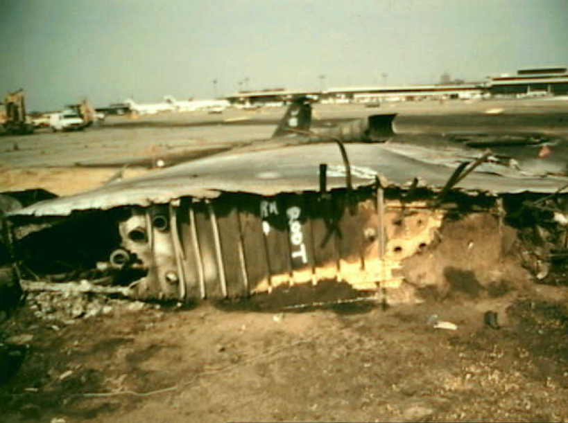
Structures 7 - Photo 9. View looking outboard of right wing at the separated wing root
