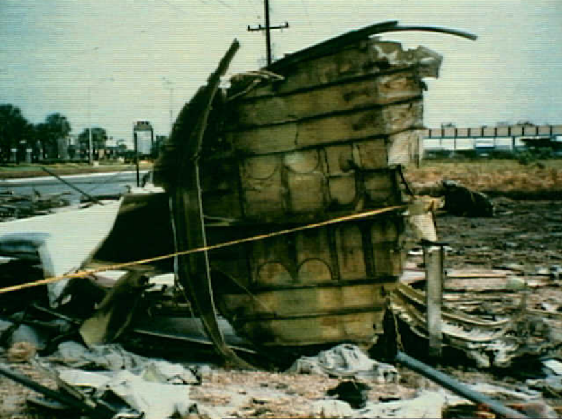
Structures 7 - Photo 7. View of the vertical stabilizer and aft pressure bulkhead.
