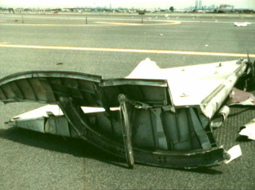
Structures 7 - Photo 7. View of the right inboard trailing edge wing flap
