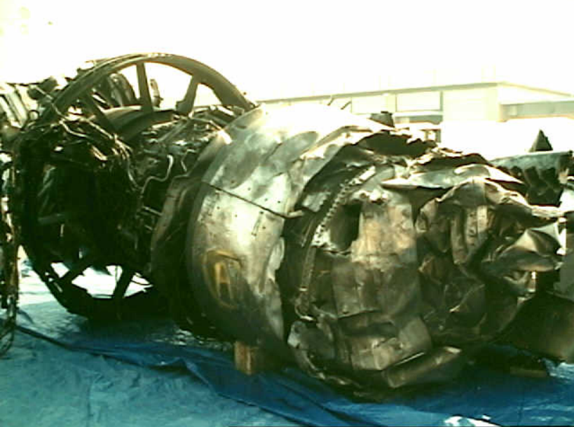
Structures 7 - Photo 6. View of the No. 3 (right) engine Note: engine tail cone is crushed and the engine inlet case is destroyed
