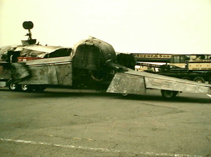
Structures 7 - Photo 4. View of the empennage and damaged outboard end of the left horizontal stabilizer
