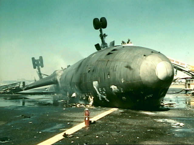
Structures 7 - Photo 3. View looking aft at the nose of the airplane Note: the nose landing gear and left main gear are extended and the fuselage is resting on it's left wing
