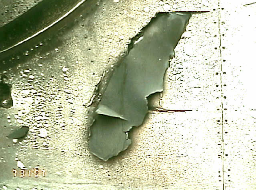
Structures 7 - Photo 23. View of engine fan blade embedded in the left side of the fuselage above the left
