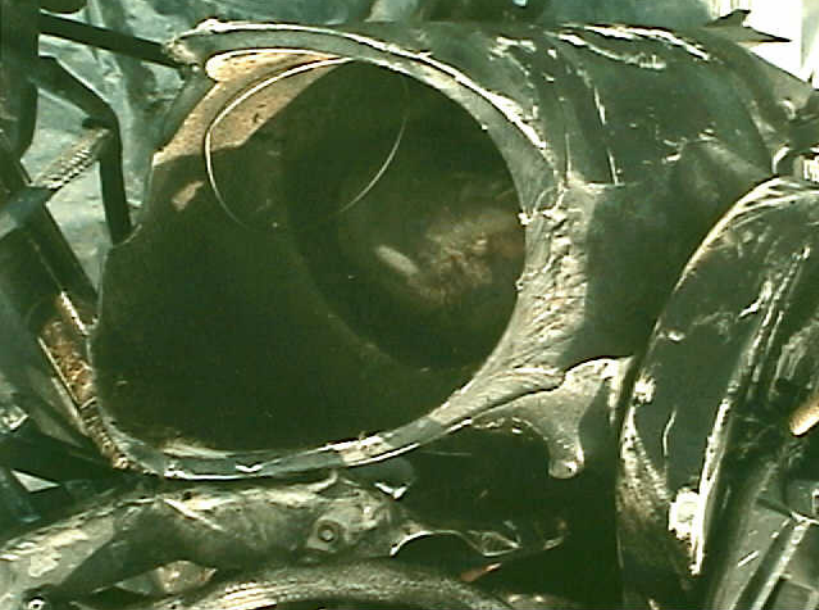
Structures 7 - Photo 21. Fractured right landing gear bogie beam
