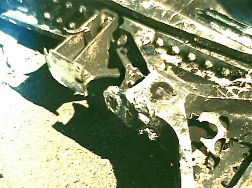
Structures 7 - Photo 19. View of fractured right landing gear trapezoidal panel
