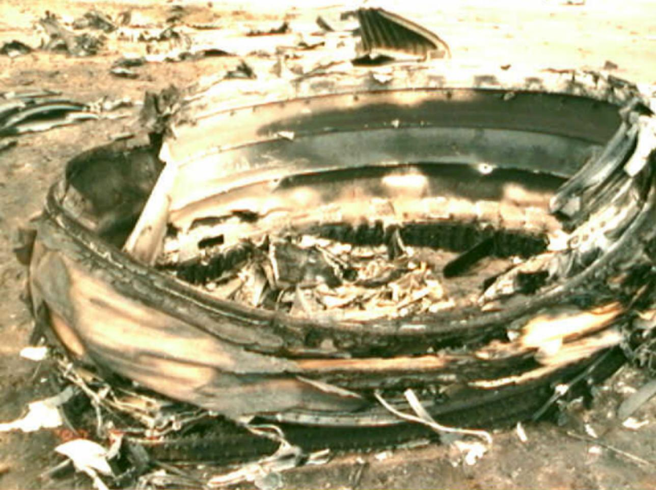
Structures 7 - Photo 17. View of separated engine inlet
