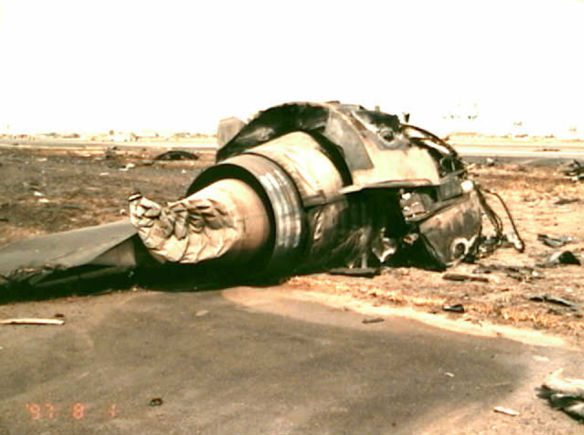
Structures 7 - Photo 15. View of No. 1 (left) engine and engine pylon
