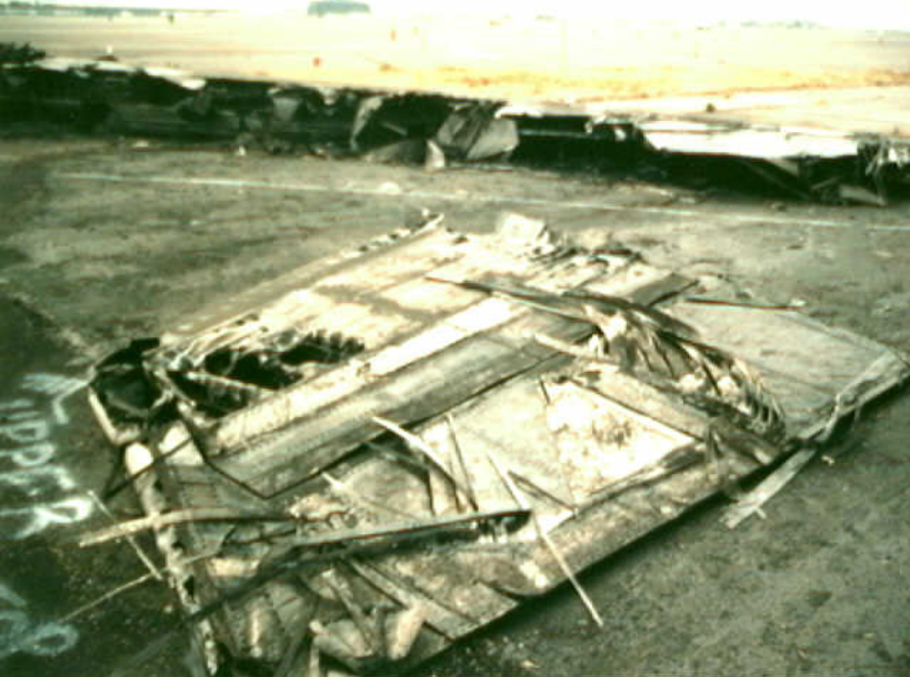
Structures 7 - Photo 14. View of burned outboard section of right horizontal stabilizer
