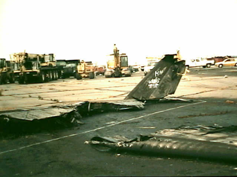
Structures 7 - Photo 13. View of outboard right wing tip and outboard section of right horizontal stabilizer in foreground. Note: lower winglet is separated from the outboard wing
