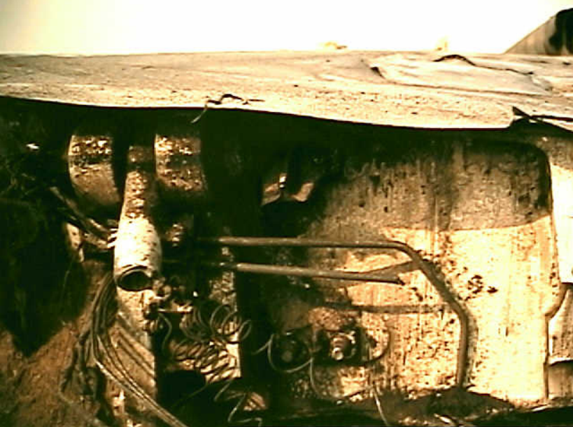
Structures 7 - Photo 11. View of fixed brace, forward and aft mounts for the right landing gear
