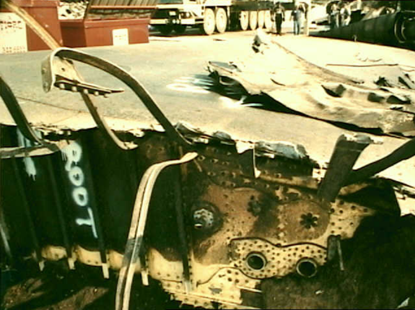
Structures 7 - Photo 10. Close-up view of right wing Note: fractured stringers bent upwards
