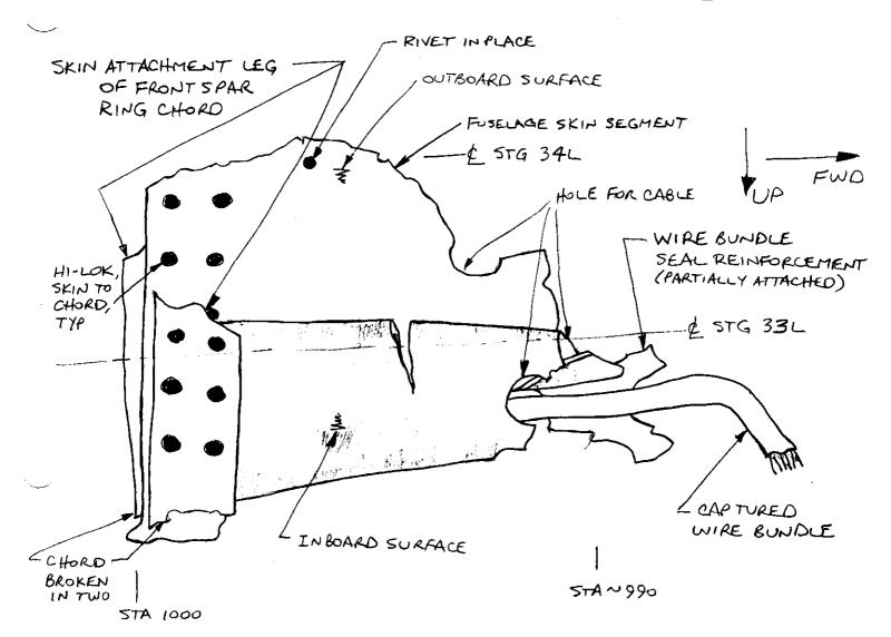
SKIN IS DRAMATICALLY COILED WITH VARIABLE OUTSIDE RADII. AT STA 1000 THE CURVE RADIUS IS ABOUT 1/2 INCH. AT STA-990 THE CURVE RADIUS IS ABOUT 1 INCH.
