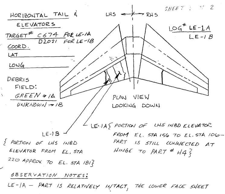
IS BROKEN BTWN ELSTA 119 & 106 - SEE SKETCH, THE LOWER SURFACE IS STREAKED, EWAS OF TYPICAL APPEARANCE PER CONSULTATION WITH TWA MECHANIC, DUE TO HYDRAULIC FLUID OR GREASE LEAKING ON TO SURFACE } NO OBVIOUS SIGNS OF FIRE DAMAGE. THERE IS ONLY VERY LIGHT SOOTING IF ANY ON PART,
