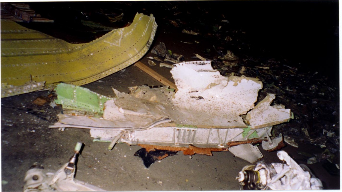
Photo #7 - Inboard Main Flap Box
