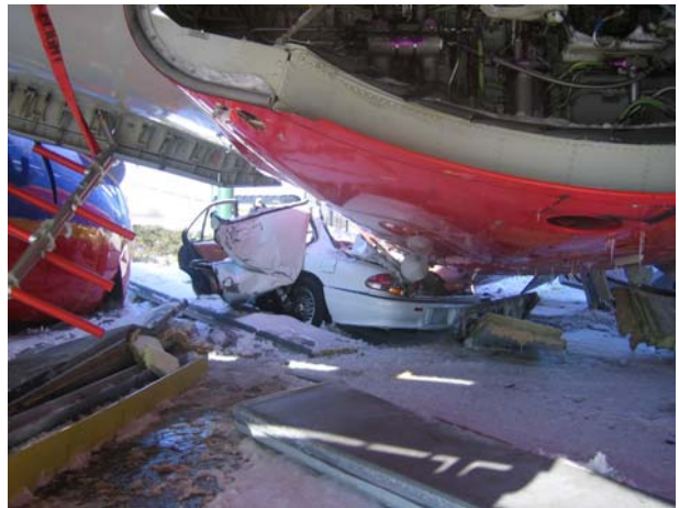
Figure 4. "As-found" relation of airplane and Pontiac.
