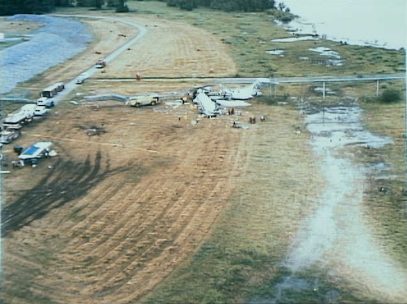
Structures 7 - Exhibit No. 7C - Photo 9. View of the forward and center fuselage sections. Note the crushing damage to the fuselage nose and the lighting system structure (i.e. angles) protruding from the fuselage near the forward galley service door.
