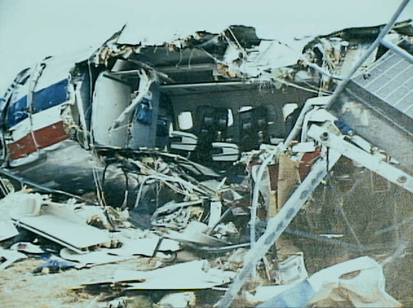
Structures 7 - Exhibit No. 7C - Photo 15. View of the left (aft) overwing emergency exit door external surface near its respective opening. Note the closed position of the external door handle and the fire damage to the leading edge and lower aft corner.
