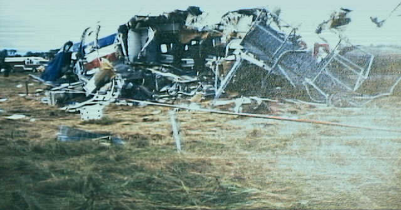
Structures 7 - Exhibit No. 7C - Photo 14. View of the rear fuselage from beneath the runway 22L approach lighting system catwalk. Note the extensive heat damage (i.e. sagging skin) on the upper fuselage shell, forward of the rear pressure bulkhead.
