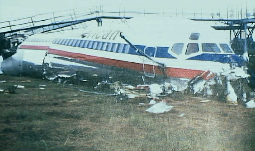
Structures 7 - Exhibit No. 7C - Photo 13. View of the rear fuselage and right wing. Note the passenger cabin and upper fuselage consumed by fire. Note the detached landing gear and inboard section of the inboard flap immediately aft of the wing..
