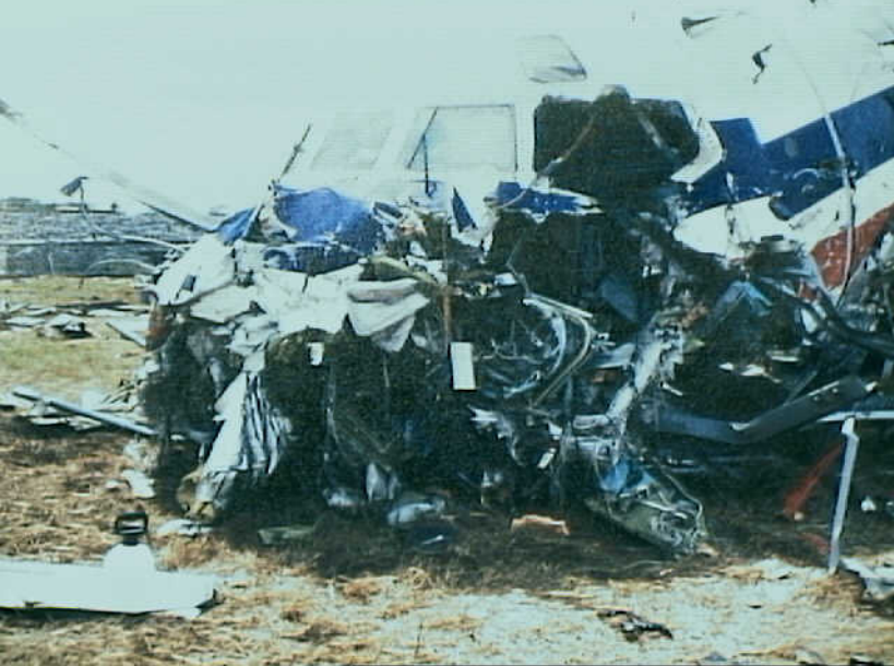
Structures 7 - Exhibit No. 7C - Photo 12. View of the rear fuselage and separated left wing. Note the extensive fire damage to the passenger cabin. Also note the lighting system structural support column obstructing the aft galley service door opening.
