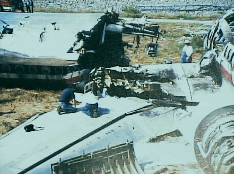
Structures 7 - Exhibit No. 7C - Photo 11. Close up view of the forward fuselage, left side. Note the extensive damage to the flooring and underlying airframe structure. Note that the first class seats on the left side are completely missing. (NTSB)
