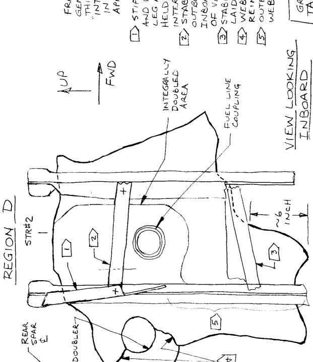
FRACTURE LINES OF WEB GENERALLY "CLEAN-CUT" IN THINNER AREAS BUT EXHIBITS INTER-LAMINAR" SHEARING IN THICK REGIONS. NO APPARENT CHARRING. AND WEB SEPARATED FROM LEG ATTACHED TO WEB, BUT HELD IN PLACE BY STABILIZATION INTERCASTAL [2).
