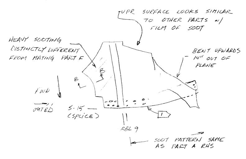
FAILURE BY STR SEVERING ALL FRACTURE SURFACES FREE OF BLACKENING
