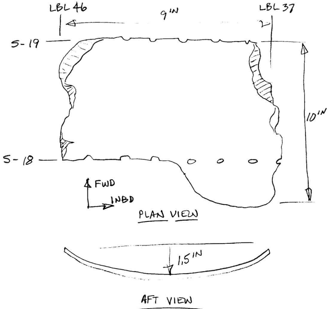
NO SOOTING APPARENT, ALL FRACTURES DUCTILE.
