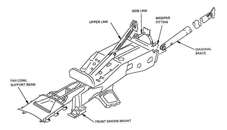
Figure 1. Engine Pylon Diagram
