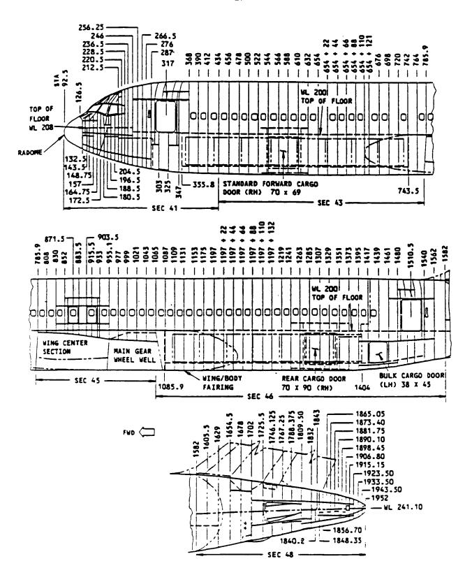
Figure 1. Fuselage Stations
