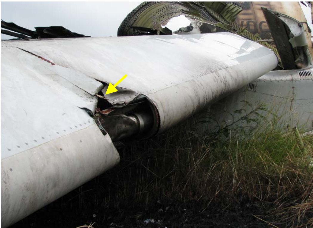
Figure 11 – Slat 2 damage with embedded wood fibers
