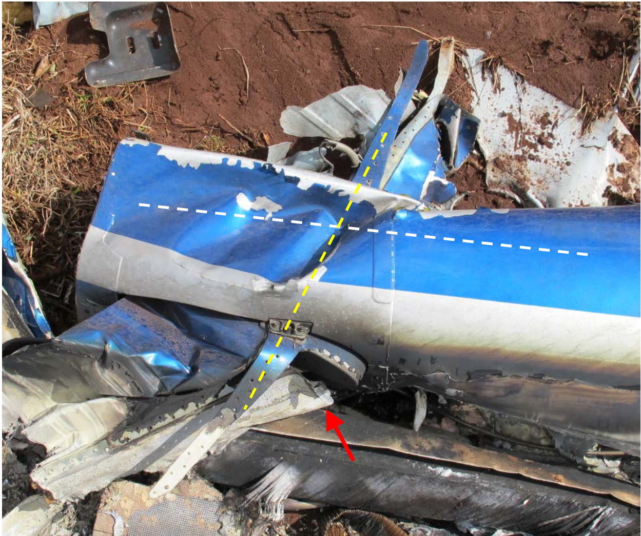
Figure 6 – Horizontal stabilizer deformation in tailboom as found at impact site
