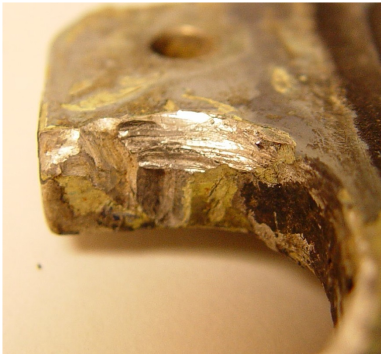
Figure 24 - Damage to upper, forward edge of right, lower stabilizer fitting
