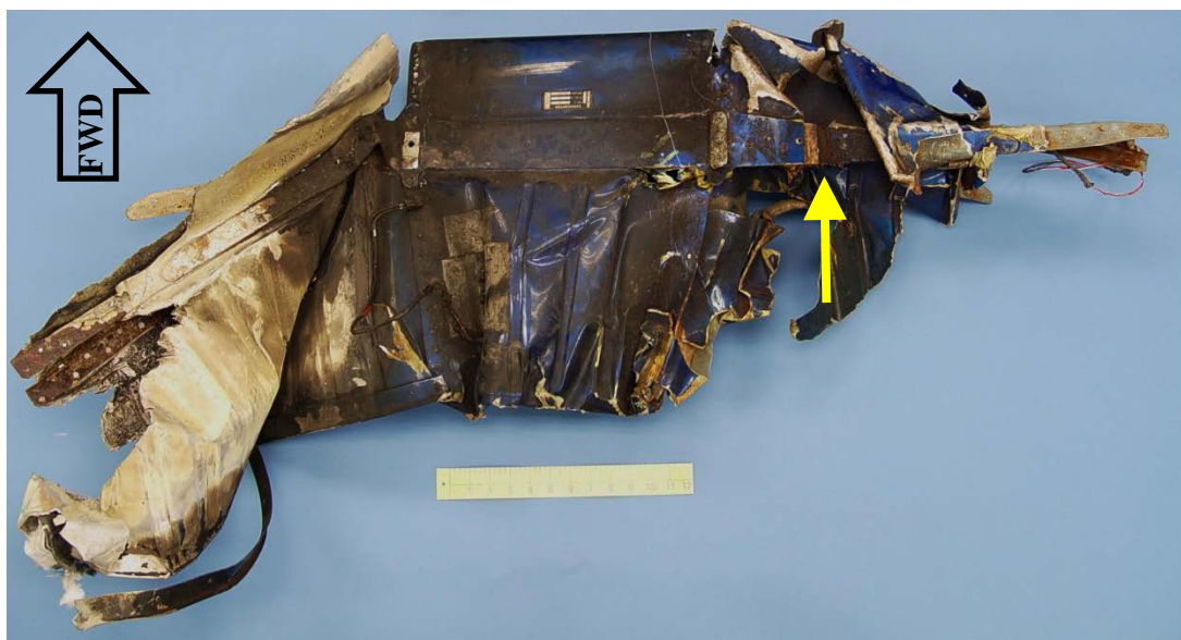
Figure 8 – Horizontal stabilizer after disassembly, top view
