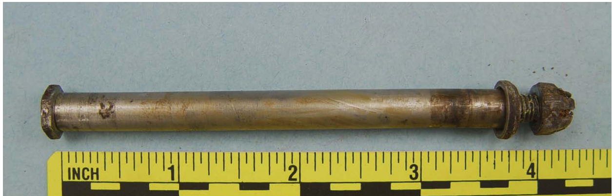
Figure 15 – Left stabilizer attach bolt
