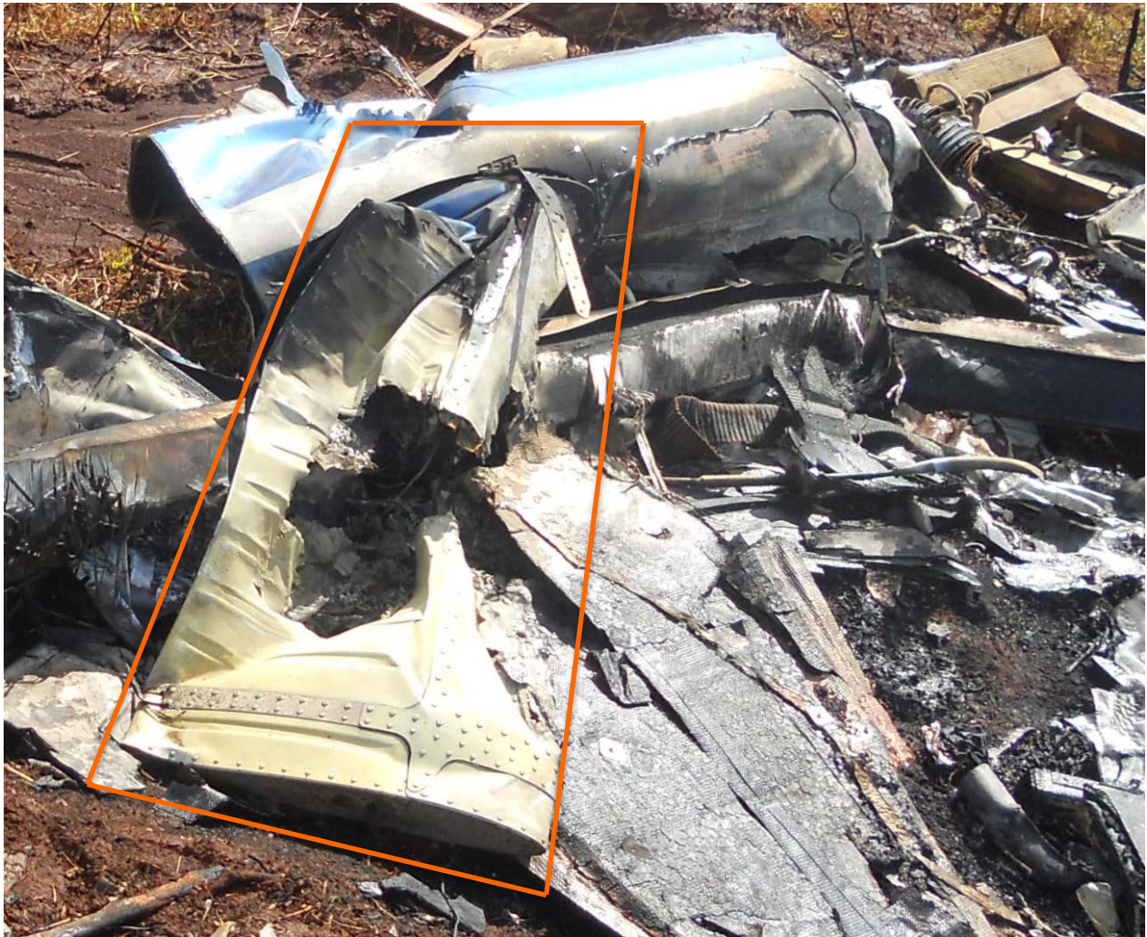
Figure 5 – Aft section of tailboom and left horizontal stabilizer as found at impact site
