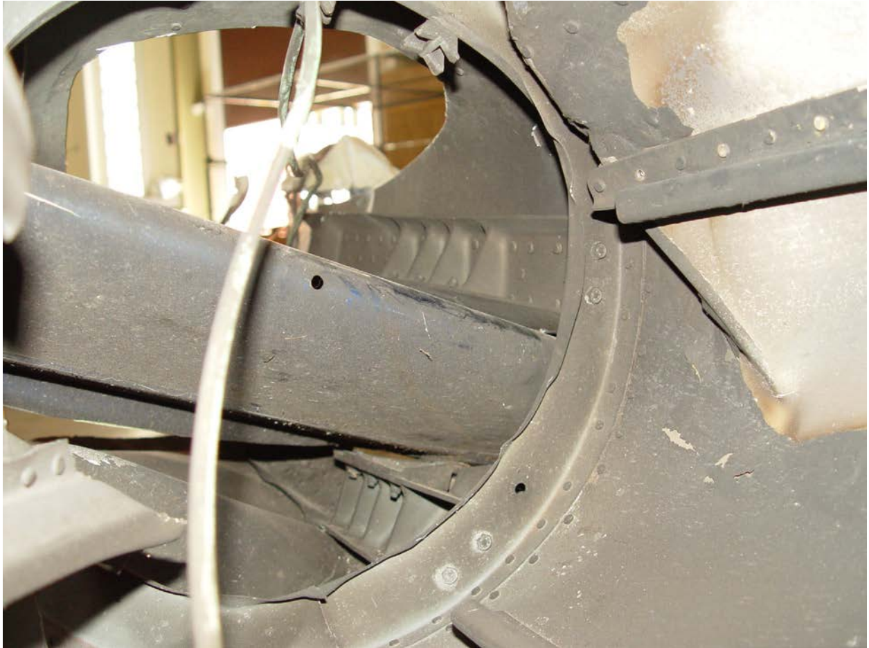
Figure 27 – Left side of ring frame at left forward longeron attach points, looking aft
