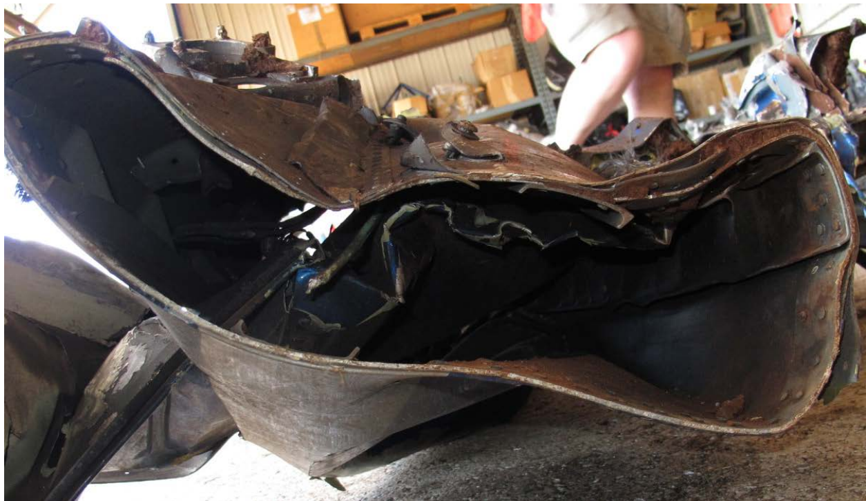
Figure 26 – Aft end of tailboom at junction frame fracture, looking forward
