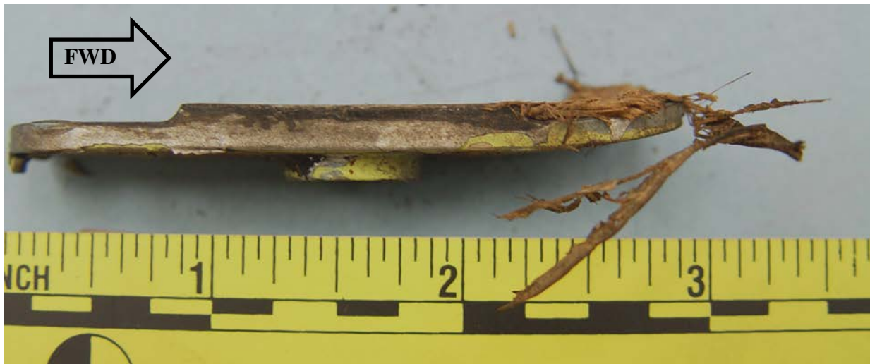
Figure 18 – Right, lower shim and wood debris
