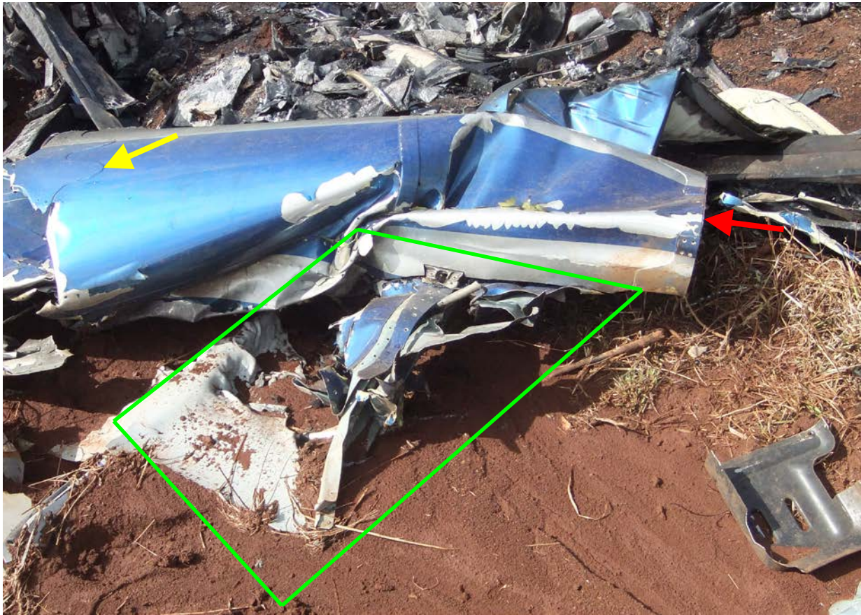
Figure 4 – Aft section of tailboom and right horizontal stabilizer as found at impact site
