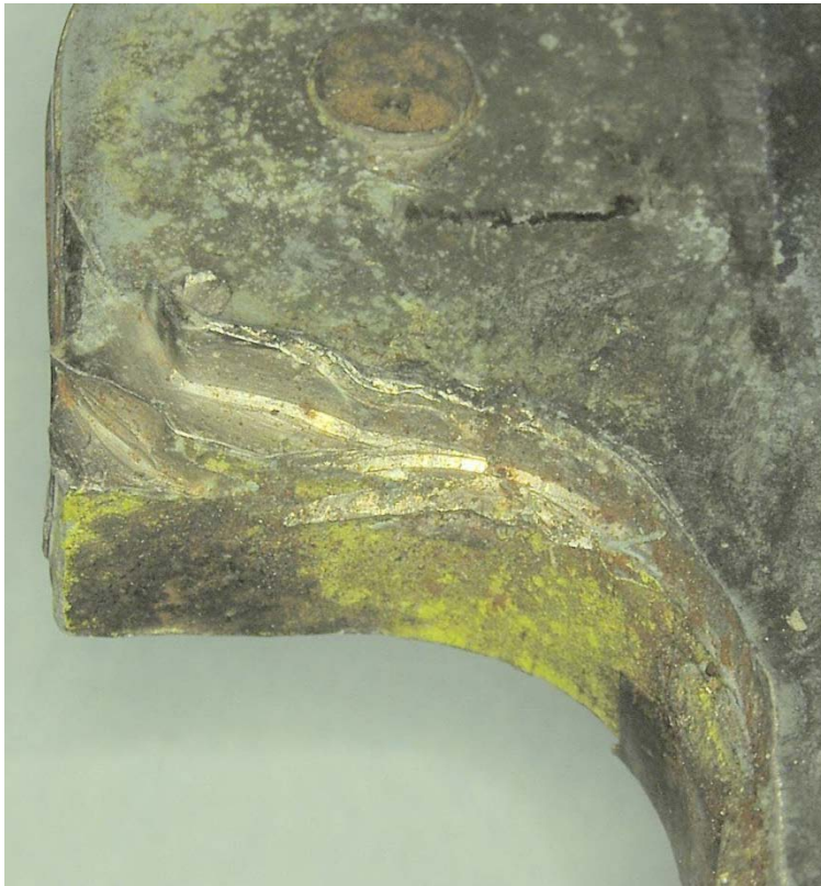
Figure 21 – Damage to lower, forward edge of right, upper stabilizer fitting
