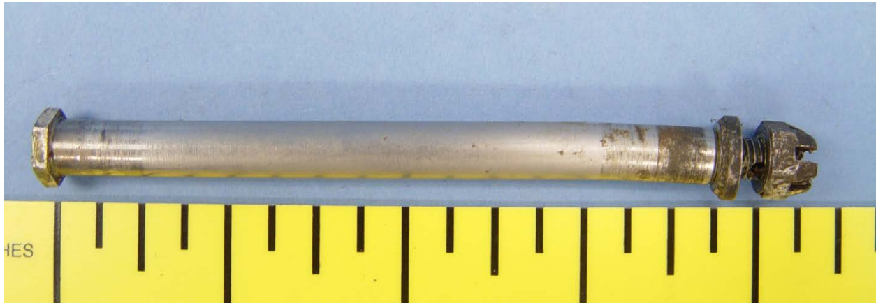
Figure 25 – Right stabilizer attach bolt
