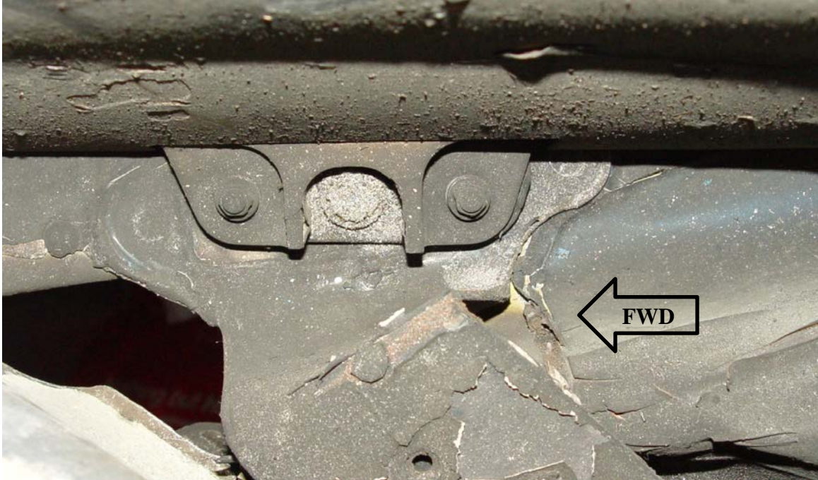
Figure 11 – Left, upper stabilizer attach point
