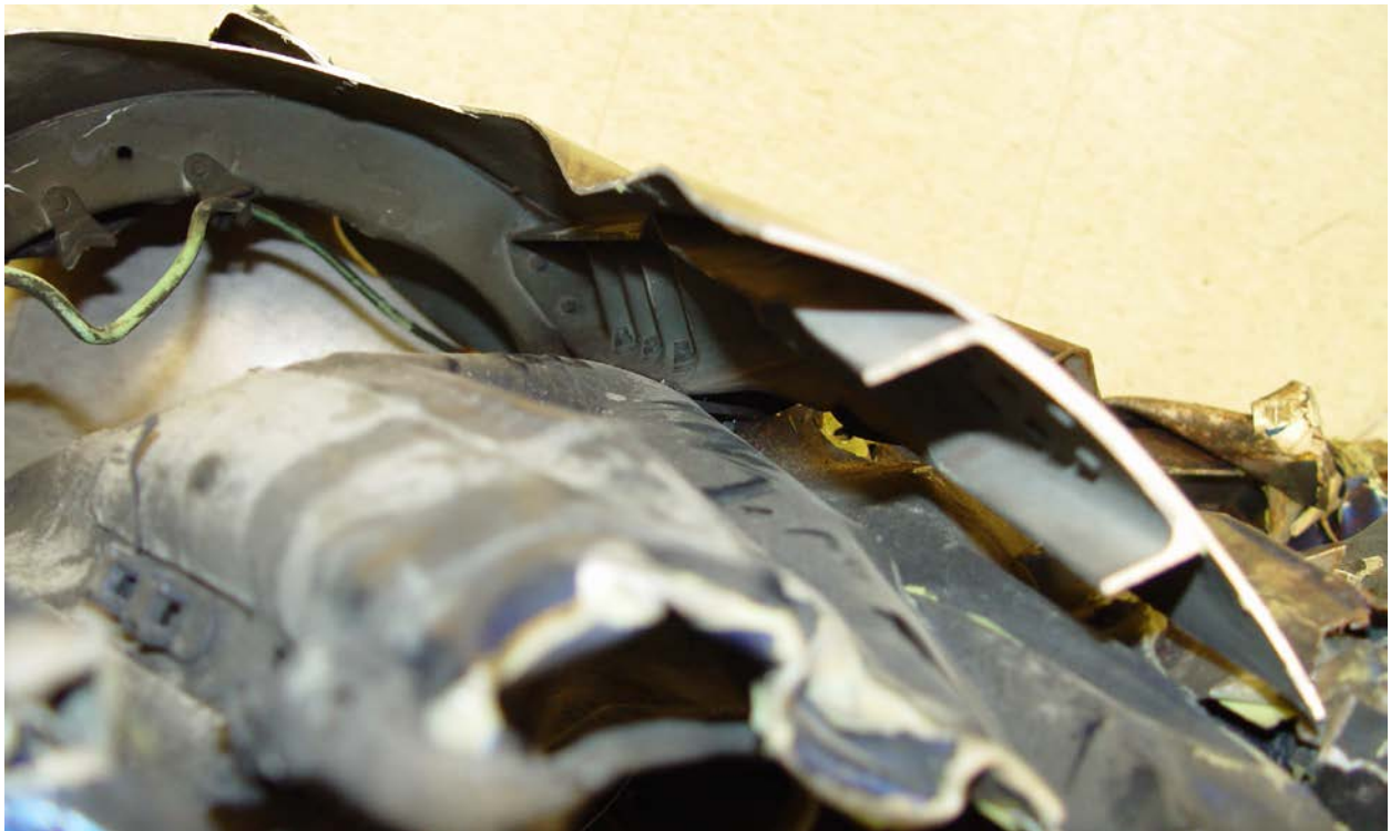
Figure 30 – Right, upper longeron, looking forward
